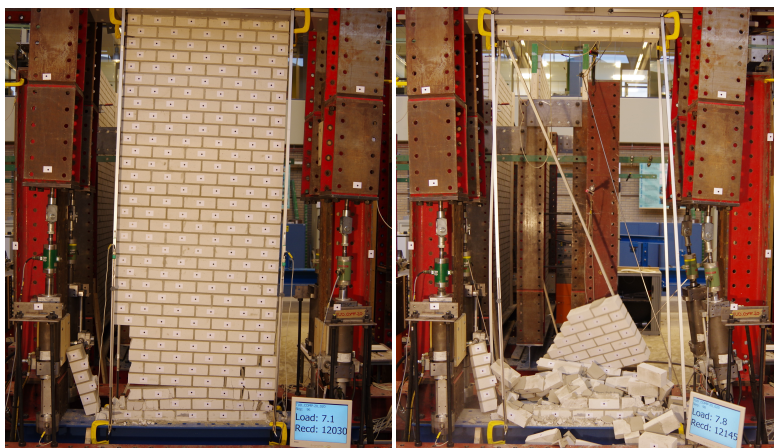
Figure 4.4: Failure pattern of masonry wall in the TUDCOMP20 experiment before collapse (left) and after collapse (right) [48]
