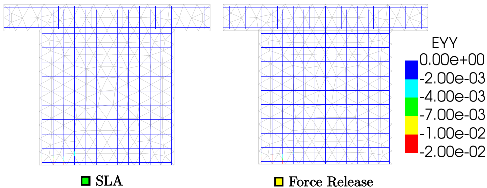
Figure 4.10: Reinforcement vertical strain patterns of SLA & Force-Release simulations of the RC shear wall experiment indicating compressive yielding and rupture (at the toe region) at the onset of collapse (refer Figure 4.8)
