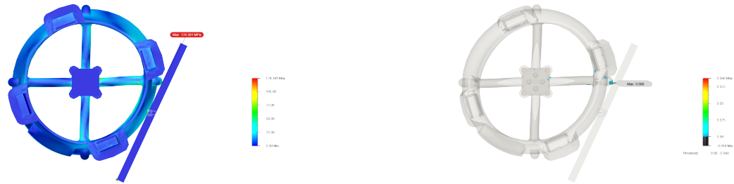
(a) Maximum stress of \sigma = 124.391 MPa at t = 0.56 ms (step 14/25) - bottom view. (b) Plastic strain at t = 1 ms (step 25/25). The mean plastic strain equals 0.001463, and 111/76914 (0.144%) elements have yielded.
