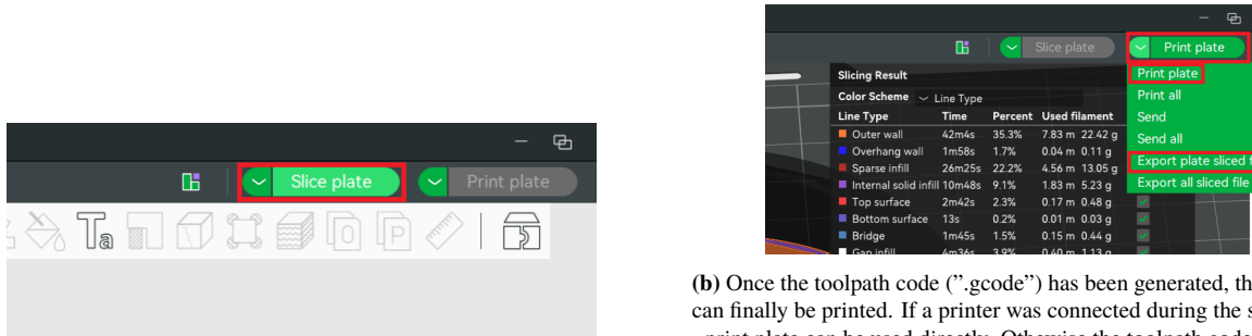
(a) To generate the machine toolpath code (".gcode") press slice plate at the top right corner
