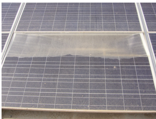
Figure 1.5: A PV module with extreme delamination where the back half of the encapsulant has separated from the glass [59].
