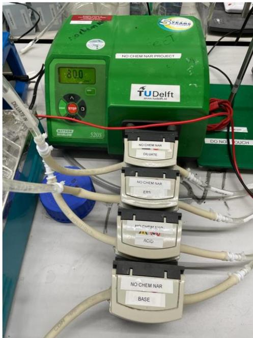
Fig. 1.2: Pump with pump heads of each compartment
