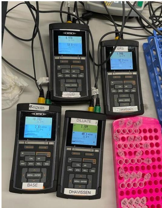
For pH, WTW Multi 3620 IDS multimeters, and for EC, WTW Multi 3620 IDS multimeters.
