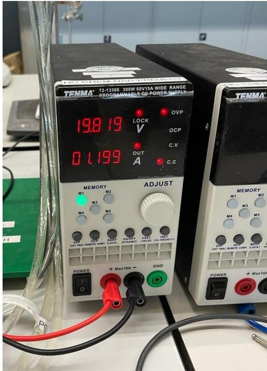
The electric current and potential were applied using a TENMA 72-1330 power supply box.
