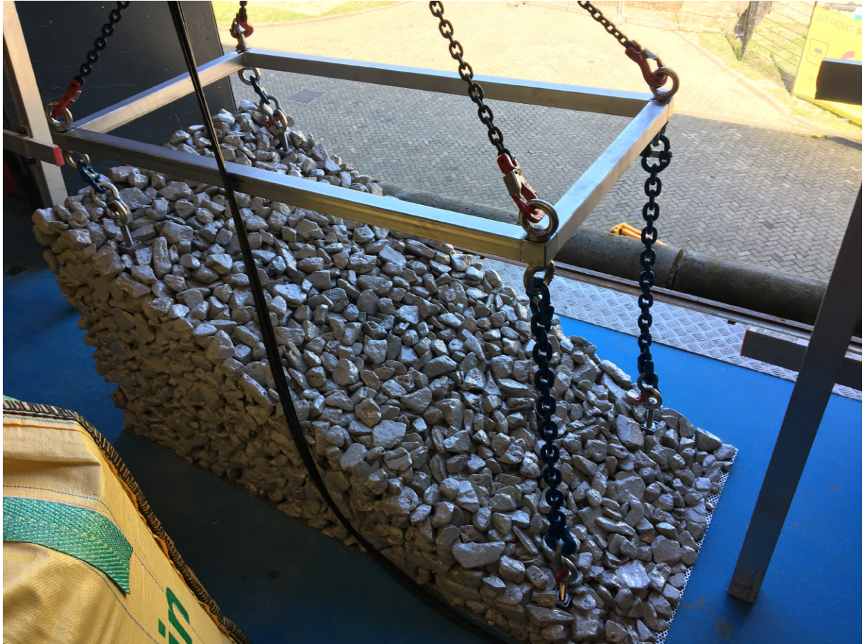
Figure C.3: Rigid breakwater while hanging in crane
