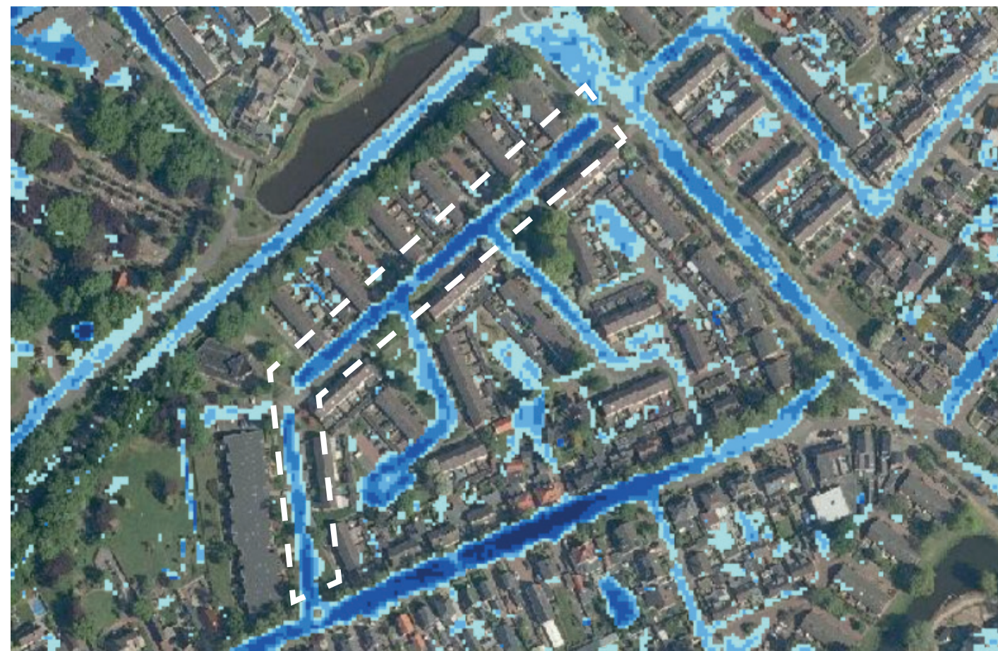
Water depth during heavy rain. 70mm - 2 hours (Klimaat-effectatlas, 2023)
