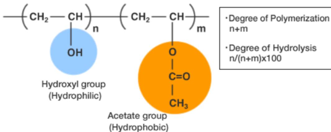
Figure 21 Structure of PVA, resulting from the partial hydrolysis of polymerized vinyl acetates. Both the degree of polymerization and the degree of hydrolysis are shown with  $n$  = the number of vinyl alcohol monomers and  $m$  = the number of vinyl acetate monomers. Retrieved from <http://www.j-vp.co.jp> September 23, 2018.
