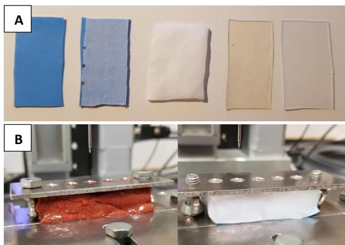
Fig. 2. (A) Samples of blood vessel mimicking materials used for needle insertion experiments. From left to right: Smooth-Sil 950 silicone, Smooth-Sil 950 silicone with mesh fabric, PVA (7m%, 4 freeze-thaw cycles), PMC-780 Dry PU-rubber, Dragon Skin 20 silicone. (B) Samples used for force profile experiments. Left: 15 mm layer of liver tissue with liver vein attached. Right: 15 mm layer of PVA with silicone and mesh fabric attached.
