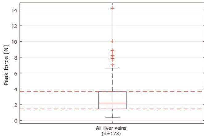
Fig. 5. Boxplot of the peak forces of the measurements of all portal veins and hepatic veins combined. The red dotted lines show the range of the desired peak forces for the blood vessel mimicking material.
