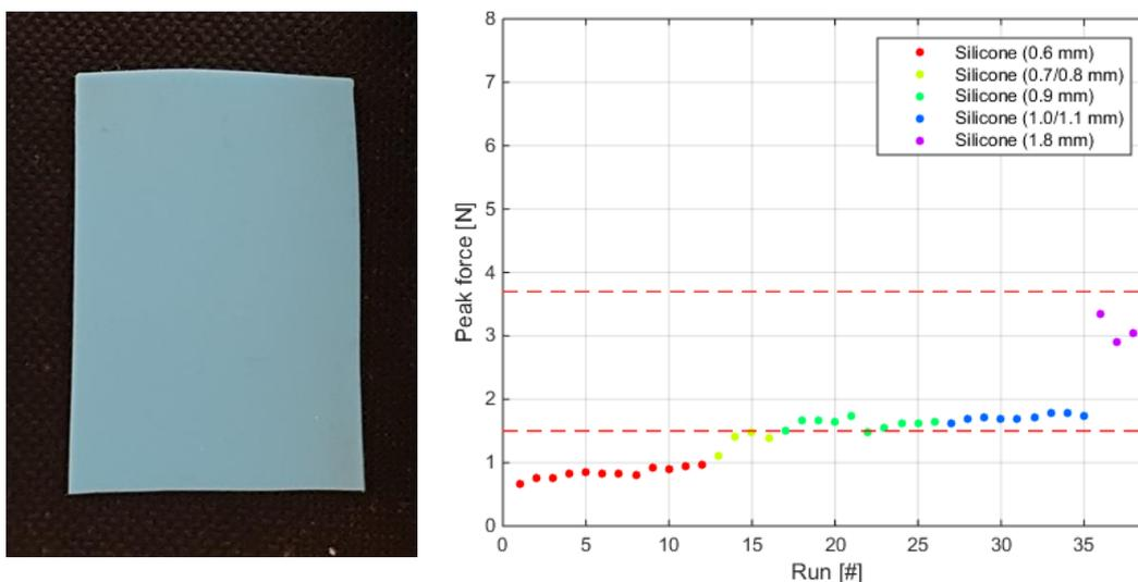
Figure 26 (Left) Sample of Smooth-Sil 950 silicone. (Right) Results of the experiments using Smooth-Sil 950 silicone samples with different thicknesses.
