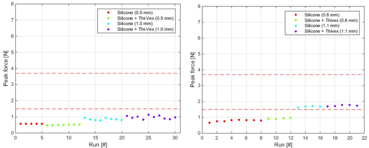
Figure 64 Influence of Thi-Vex on the peak forces for the Dragon Skin 20 silicone (left) and the Smooth-Sil 950 silicone (right).
