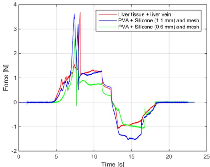
Fig. 9. A typical example of the force profiles of needle insertions into human liver samples and phantom samples. The human liver samples consist of a 15 mm layer of liver tissue with a single liver vein wall attached. The phantom samples consist of a 15 mm layer of PVA (4m%, 2 freeze-thaw cycles) with a 1.1 mm or 0.6 mm layer of silicone and mesh fabric attached.
