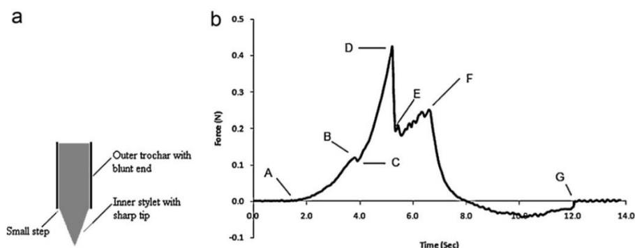
Figure 8 Typical example of needle insertion into a porcine liver. (a) Two-part needle and (b) force-time graph. Retrieved from [8].
