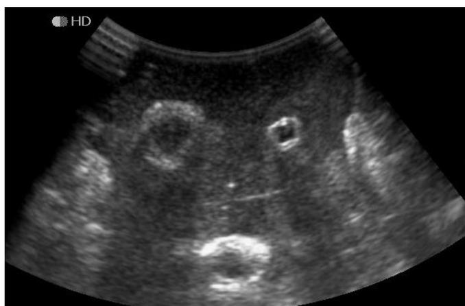
**Figure 47** Ultrasound scan of three silicone tubes with mesh embedded in PVA (4m%, 2 freeze-thaw cycles).
