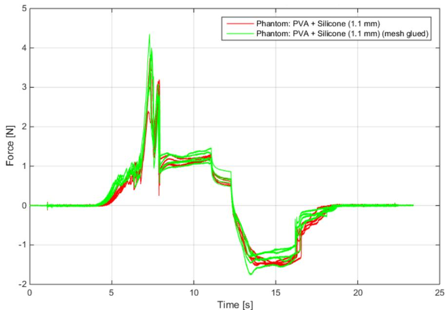
Figure 77 Force profiles of phantom samples, consisting of PVA and a 1.1 mm silicone layer with mesh fabric, both with and without glue.
