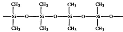
Figure 22 Structure of polydimethylsiloxane (PDMS), a common silicone. Retrieved from [63].
