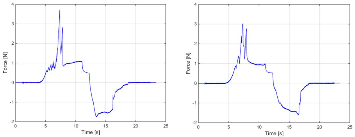
**Figure 79** Examples of force profiles of needle insertions in silicone, both with mesh fabric (left) and without mesh fabric (right).
