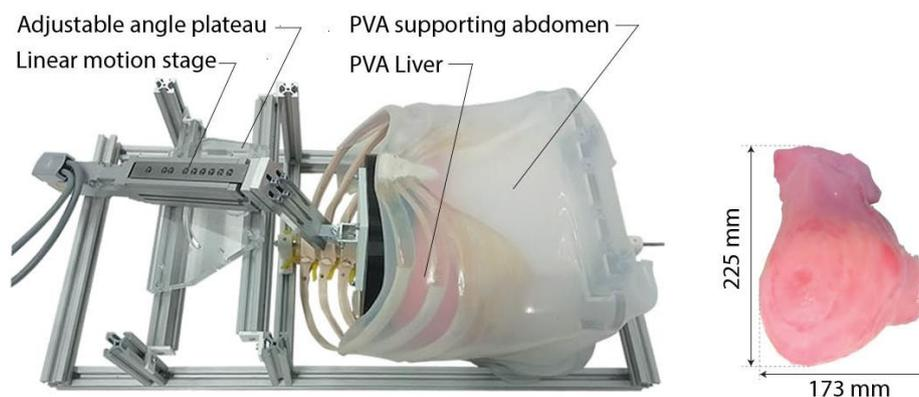
Figure 1 Setup of the PVA liver phantom with respiratory motion (left) and the PVA liver (right). Retrieved from [2].
