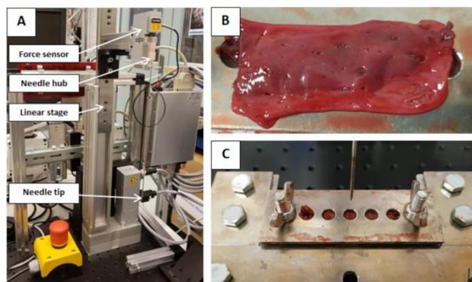
Fig 1. (A) the experimental setup, containing the force sensor and the needle, which are both mounted on the linear stage. (B) a liver vein that is retrieved from the liver and cut open. (C) a liver vein fixed between two aluminum plates and mounted underneath the needle.
