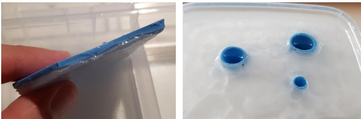
Figure 42 (Left) Bonding between a layer of silicone and mesh fabric and a layer of PVA (4m%, 2 freeze-thaw cycles).
