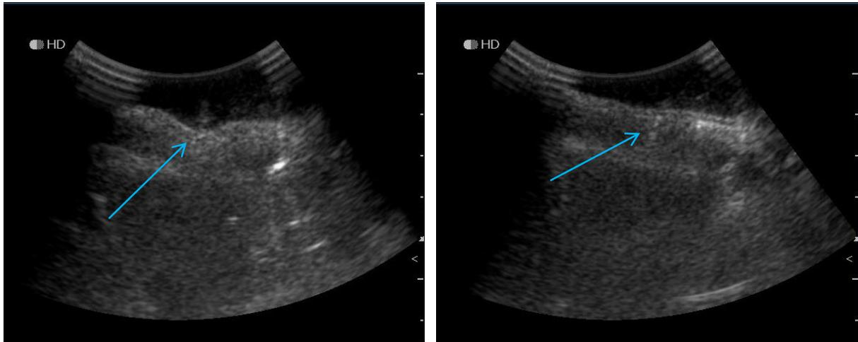
Figure 48 Ultrasound scans of a needle puncturing a silicone tube with mesh, embedded in PVA (4m%, 2 freeze-thaw cycles). Left: the needle (in-plane) makes contact with the silicone tube. Right: the needle tip (in-plane) has punctured the silicone tube.
