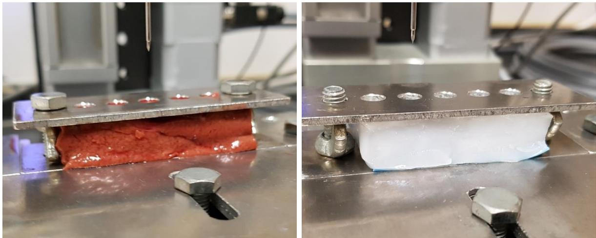
**Figure 43** Experimental setup during the force profile experiments. (Left) a 15 mm layer of liver tissue with a liver vein underneath. (Right) a 15 mm layer of PVA tissue with a silicone and mesh layer underneath.
