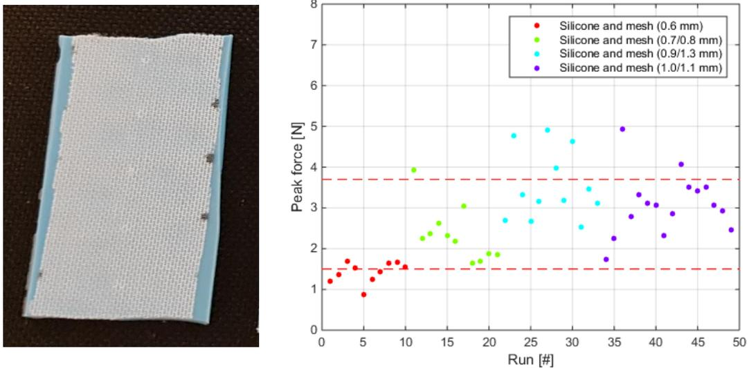
Figure 28 (Left) Sample of Smooth-Sil 950 silicone with mesh fabric. (Right) Results of the experiments using Smooth-Sil 950 silicone samples with mesh fabric and different thicknesses.
