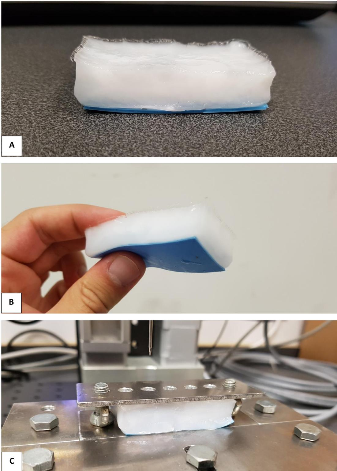
Figure 76 (A,B) Examples of the phantom samples. (C) Experimental setup for a measurement using a phantom sample.
