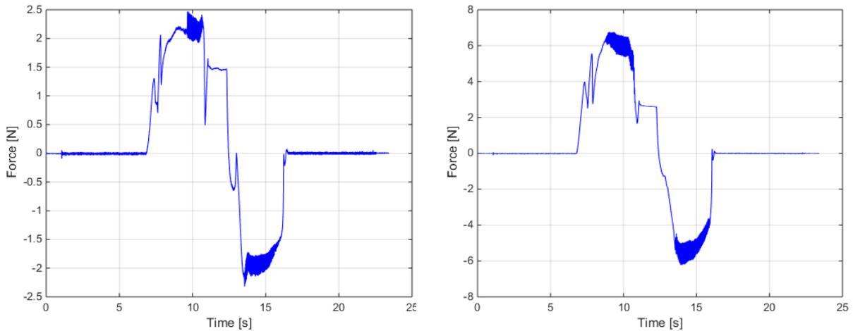
Figure 32 Force profiles during needle insertion in PMC-780 Dry PU samples, with a thickness of 0.5 mm (left) and a thickness of 1.0 mm (right).
