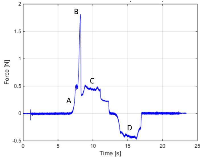
**Figure 14** A typical example of a force-time graph during a needle insertion into a blood vessel wall. At point A, the needles makes first contact with the vessel wall. Point B is the peak force during puncturing of the vessel wall. At point C the needle has punctured the blood vessel wall and the force is due to friction between the needle shaft and the vessel wall. Point D indicates the friction during retraction of the needle.
