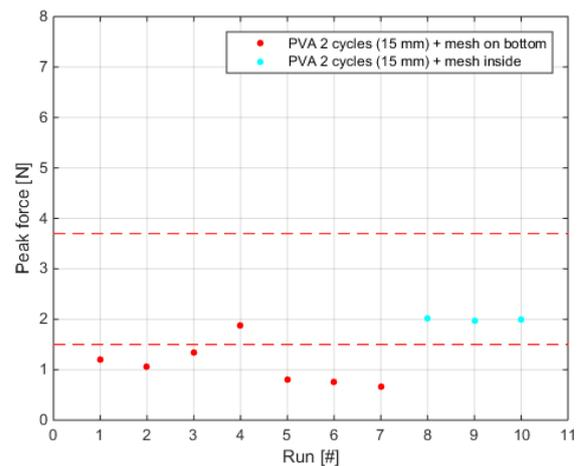
Figure 60 (Left) sample consisting of 15 mm thick PVA (7m%, 2 freeze-thaw cycles) with mesh fabric on top. (Right) results of the peak forces during needle insertions into 15 mm thick PVA with mesh fabric.
