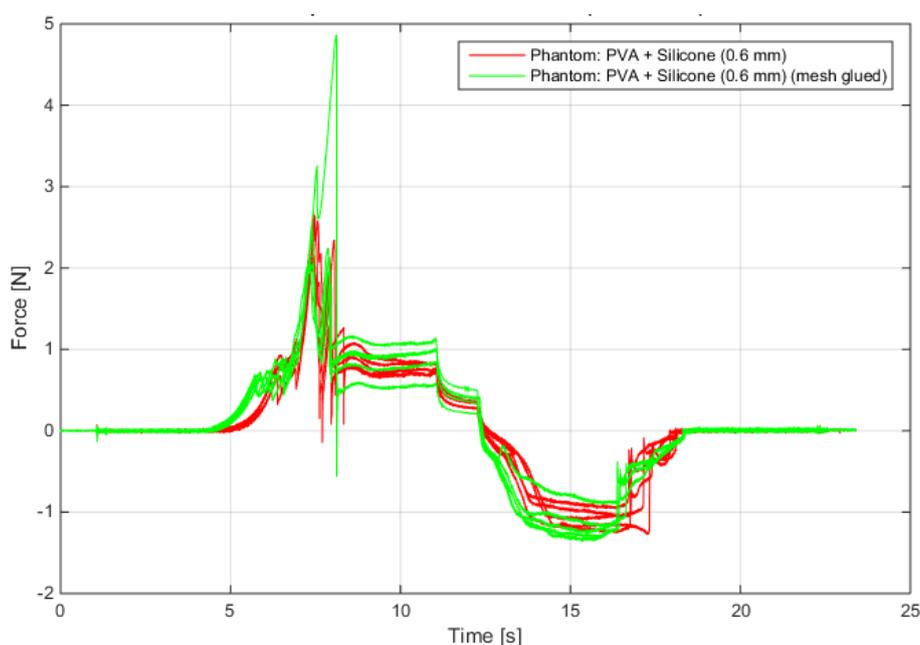
Figure 78 Force profiles of phantom samples, consisting of PVA and a 0.6 mm silicone layer with mesh fabric, both with and without glue.
