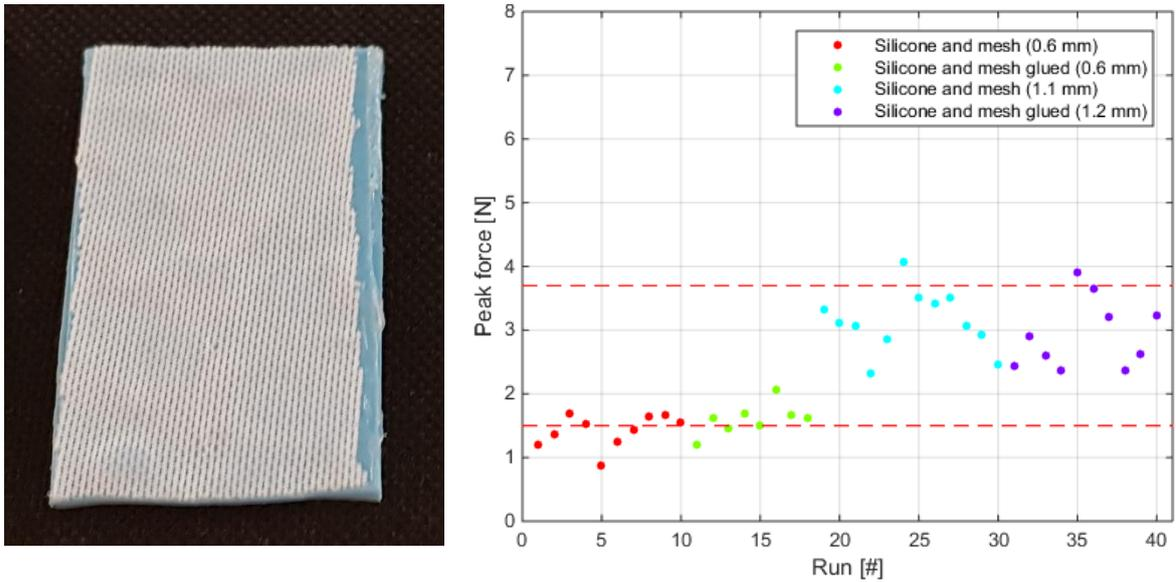
Figure 30 (Left) Sample of Smooth-Sil 950 silicone with mesh fabric. (Right) Results of the experiments using Smooth-Sil 950 silicone samples with mesh fabric and different thicknesses.
