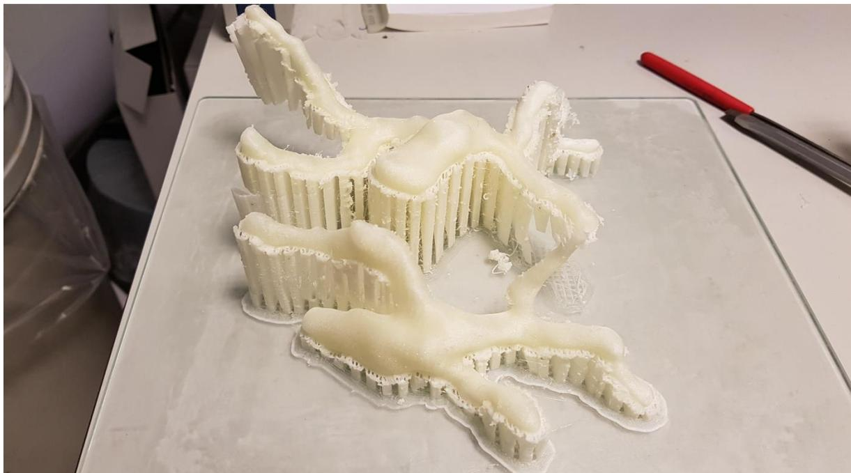
Figure 71 Results of the 3D-printed portal vein models including the support structure on the bottom.
