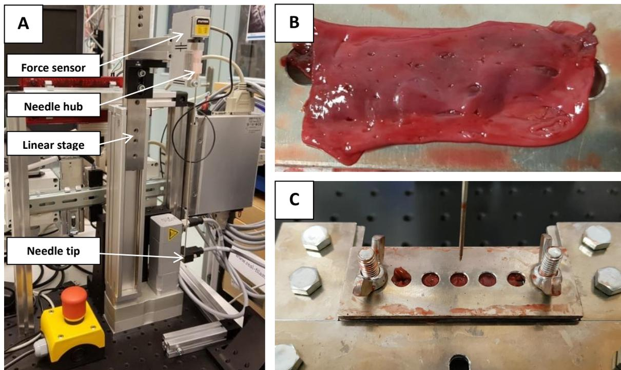
Figure 13 (A) The experimental setup, containing the force sensor and the needle, which are both mounted on the linear stage. (B) A liver vein that is cut open after it was carved out of the liver. (C) A liver vein fixed between aluminum plates and mounted underneath the needle.
