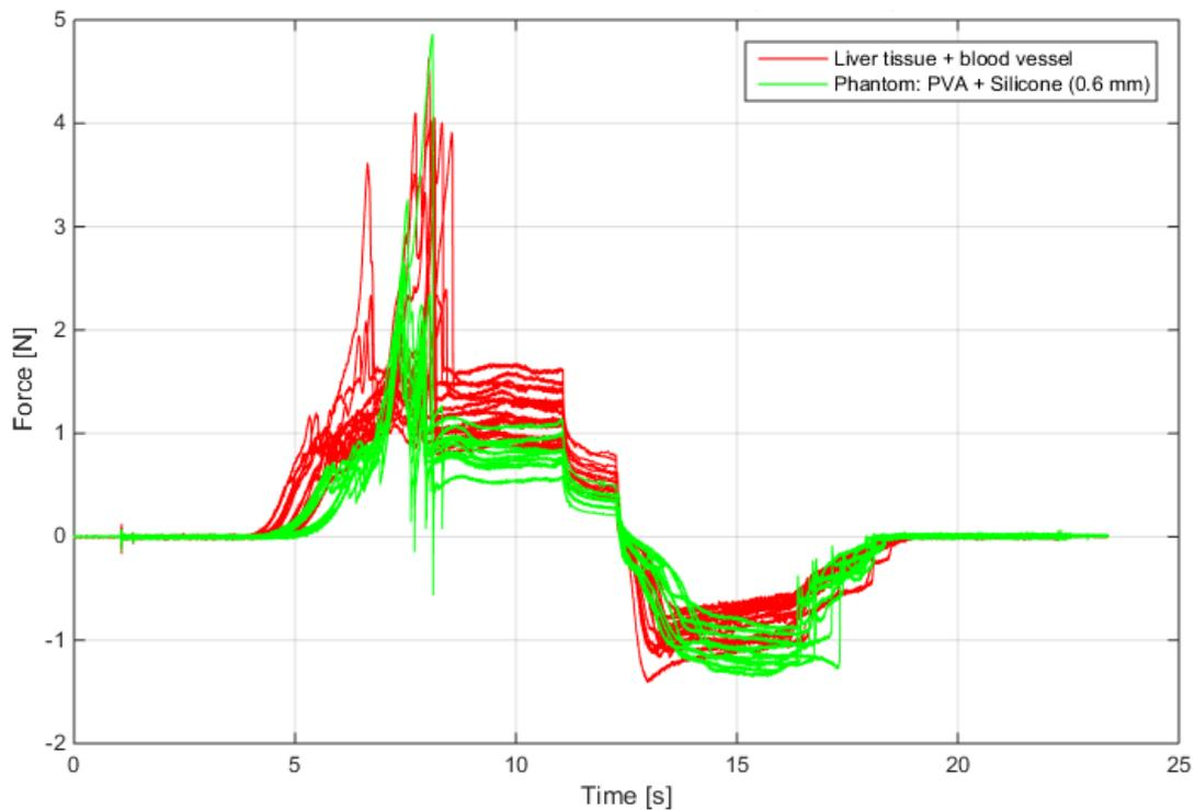
Figure 45 Force profiles of needle insertions into human liver samples and phantom samples. The human liver samples consist of a 15 mm layer of liver tissue with a liver vein attached. The phantom samples consist of a 15 mm layer of PVA (4m%, 2 freeze-thaw cycles) with a 0.6 mm layer of silicone and mesh fabric.
