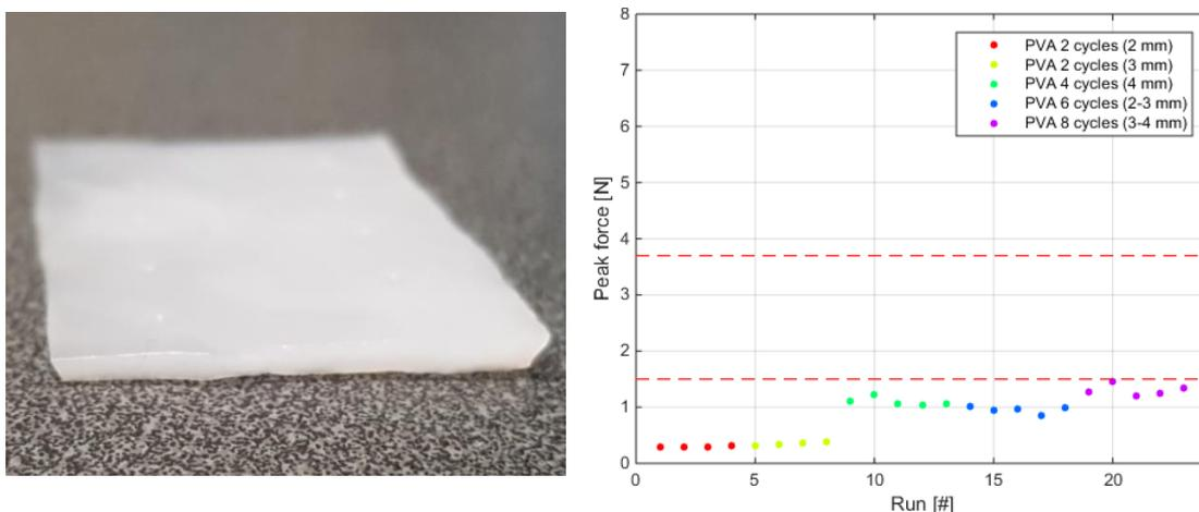
Figure 24 Example of a PVA sample (left) and the peak forces during puncturing of PVA (7m%) samples with different freeze-thaw cycles.
