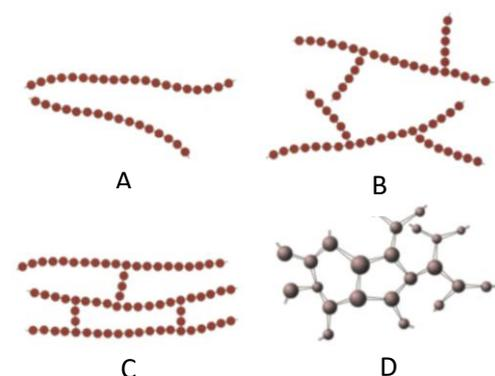
Figure 20 Different polymer structures: (A) linear, (B) branched, (C) crosslinked, (D) network. Adapted from [56].
