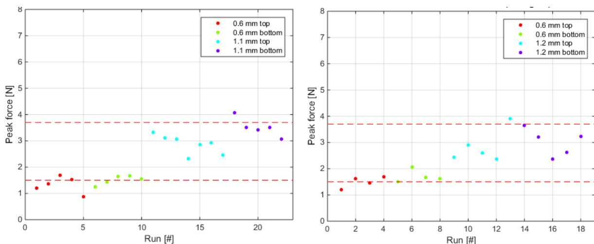
Figure 65 Peak forces during puncturing of Smooth-Sil 950 silicone samples with different thicknesses and with addition of mesh fabric. The effect of the orientation of the mesh on the peak force was examined, both without glue (left) and with glue (right).
