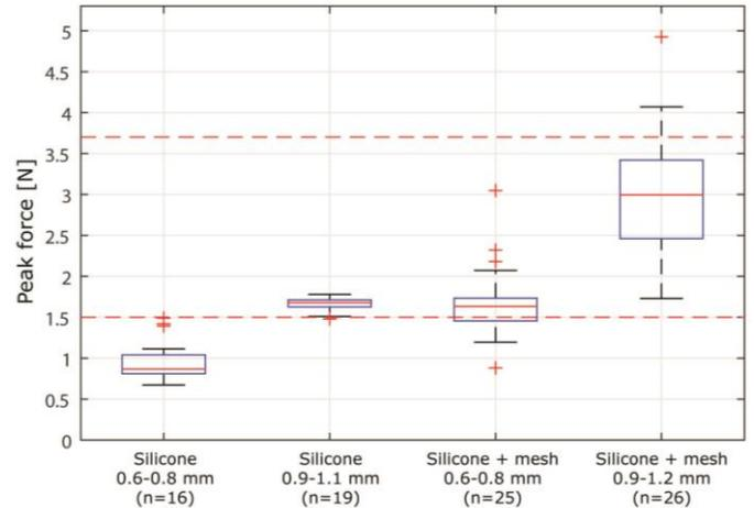
Fig. 6. Boxplot of the peak forces of Smooth-Sil 950 silicone, with and without mesh fabric, using different silicone thicknesses.
