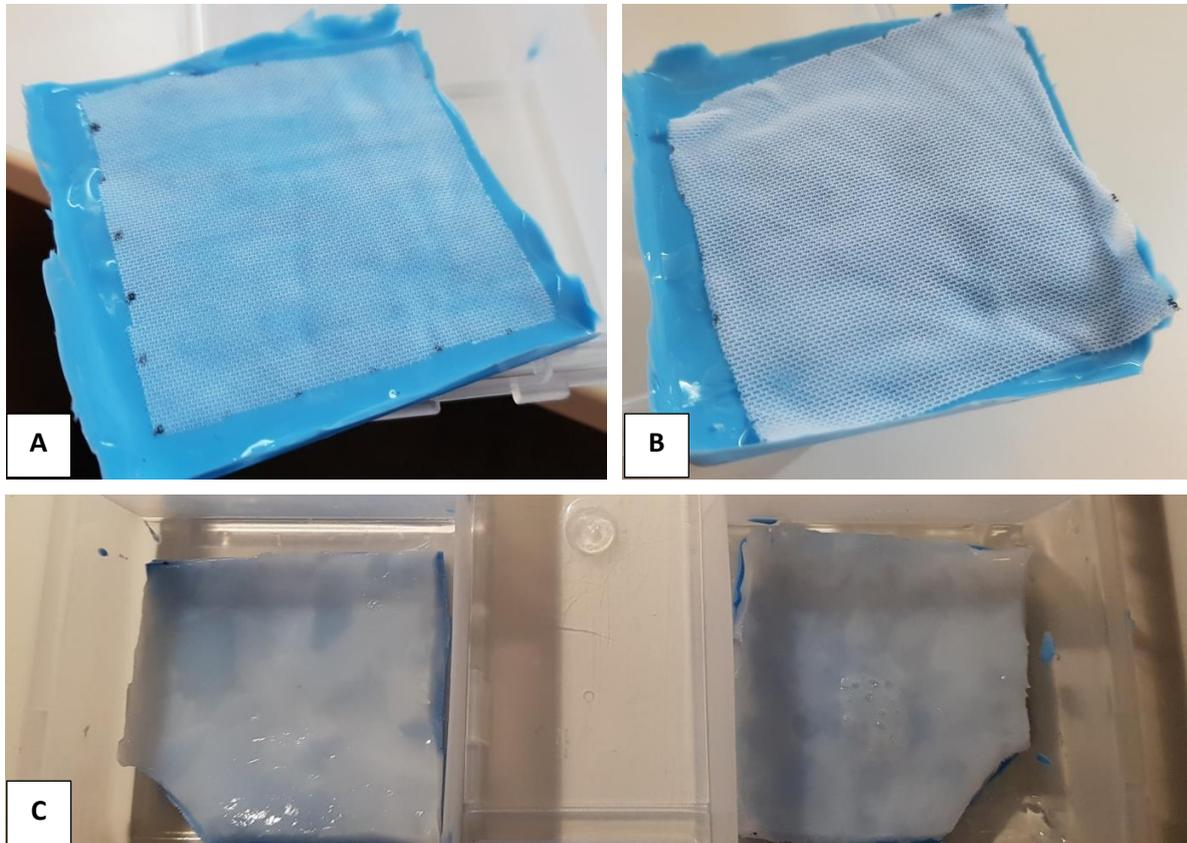
Figure 73 (A) Sample of silicone layer with mesh fabric added during hardening of the silicone. (B) Sample of silicone layer with mesh fabric glued onto the silicone. (C) Samples of PVA, silicone and mesh fabric to test bonding.
