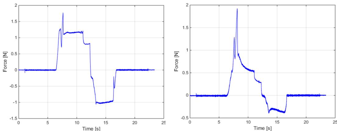
Figure 27 Force profile during needle insertion in 1.1 mm Smooth-Sil 950 silicone sample (left) and a human liver vein (right).
