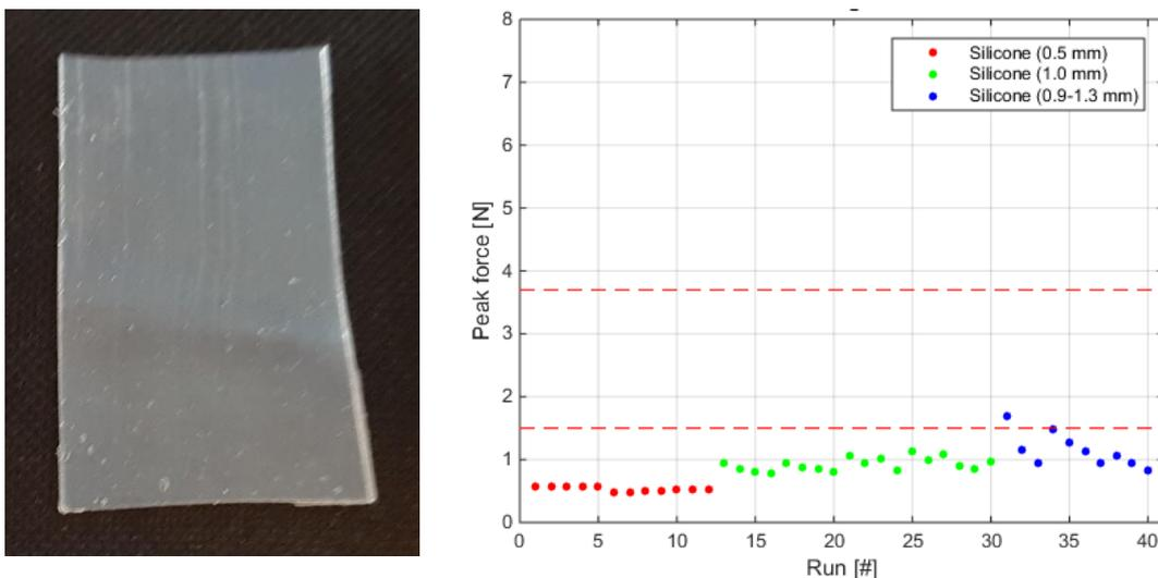
Figure 25 (Left) Two samples of Dragon Skin 20 silicone. (Right) Results of the peak forces of Dragon Skin 20 silicone with different thicknesses.
