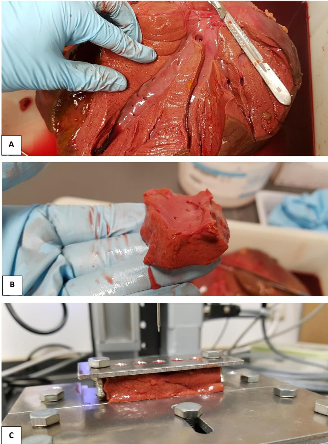
Figure 75 (A) Locating the liver vein by cutting it open. (B) Retrieval of a sample containing a liver vein and 15 mm liver tissue. (C) Experimental setup for a measurement using a human liver sample.
