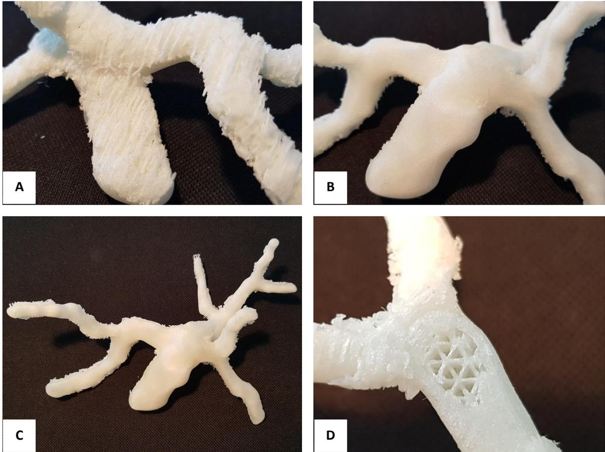
Figure 72 Details of the 3D-printed portal vein models. (A) Reminders of the support structure that are attached on the bottom of the vein model. (B) The surface on the top of the vein model. (C) The less simplified model of the portal vein, showing reminders of the support structure. (D) Part of the triangular structure inside the vein model.
