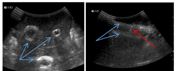
Fig. 8. Ultrasound scans of three silicone tubes embedded in PVA. The blue arrows indicate the silicone blood vessel wall and the red arrow indicates the needle tip (in-plane) after puncturing the silicone blood vessel wall.
