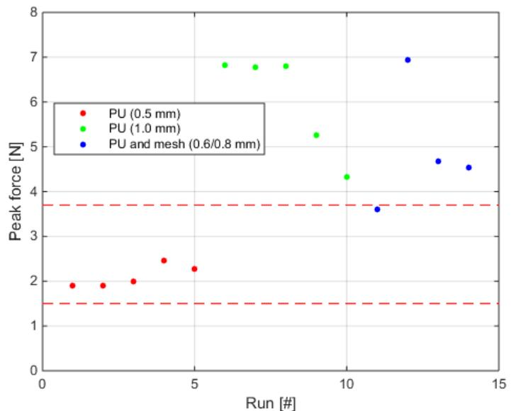
Figure 31 Peak forces during puncturing of PMC-780 Dry PU samples with different thicknesses and the addition of mesh fabric.
