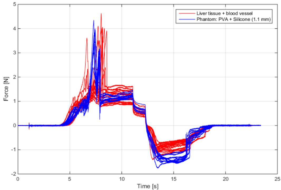
Figure 44 Force profiles of needle insertions into human liver samples and phantom samples. The human liver samples consist of a 15 mm layer of liver tissue with a liver vein attached. The phantom samples consist of a 15 mm layer of PVA (4m%, 2 freeze-thaw cycles) with a 1.1 mm layer of silicone and mesh fabric.
