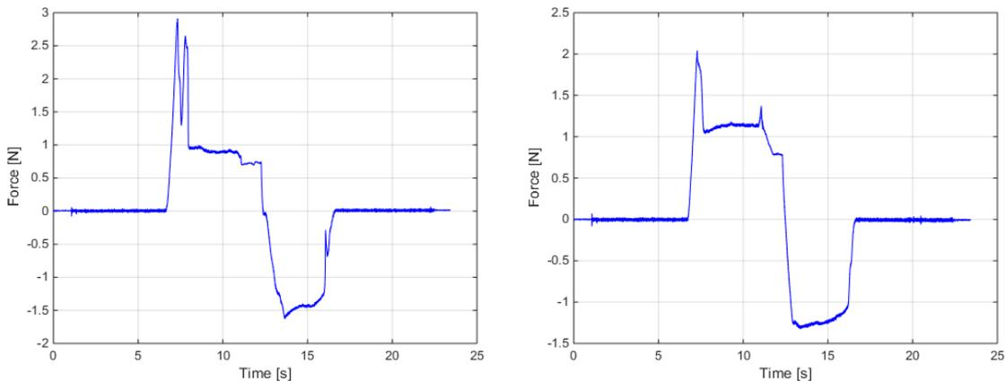
Figure 29 Force profiles during needle insertion in a 1.3 mm Smooth-Sil 950 silicone sample with mesh fabric added, with both the inner and outer needle (left) and only the inner needle (right).
