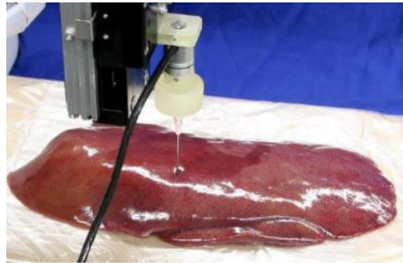
Figure 10 Experimental setup for needle insertions in porcine liver and its blood vessels. Retrieved from [11].
