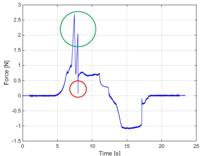
**Figure 46** Force profile of a needle insertion into a phantom sample consisting of a 15 mm layer of PVA (4m%, 2 freeze-thaw cycles) and a 0.6 mm silicone layer.
