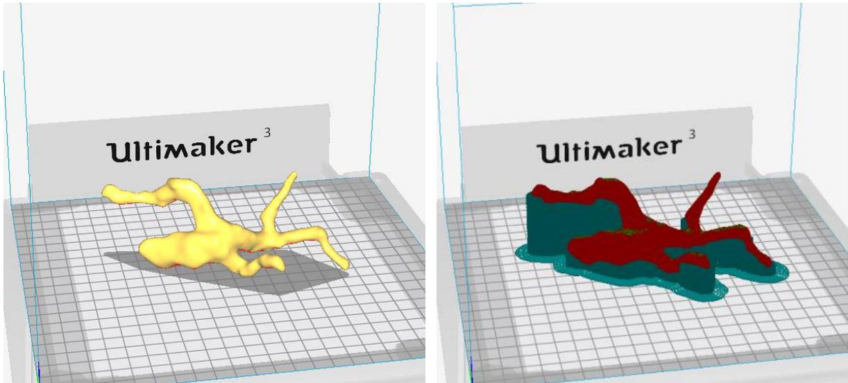
Figure 70 Simplified model of the portal vein in Cura (left). The right figure shows the portal vein model (red) and the support structure (blue).
