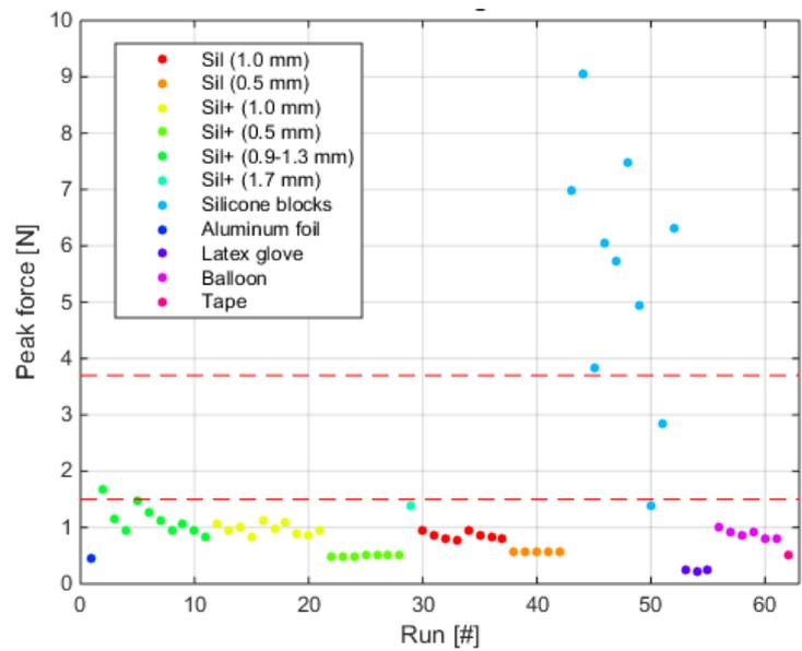
Figure 62 Peak forces during the first test using different materials. Sil indicates Dragon Skin 20 silicone and Sil+ indicates Dragon Skin 20 silicone with the addition of Thi-Vex.
