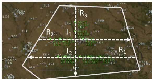
Figure 5.2: BlueSky sector with three routes R_1 , R_2 and R_3 , and two intersections I_1 and I_2 [8].
