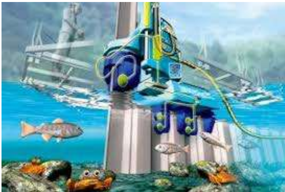
Figure 3 Seabed piling rig ( www.giken.com )
