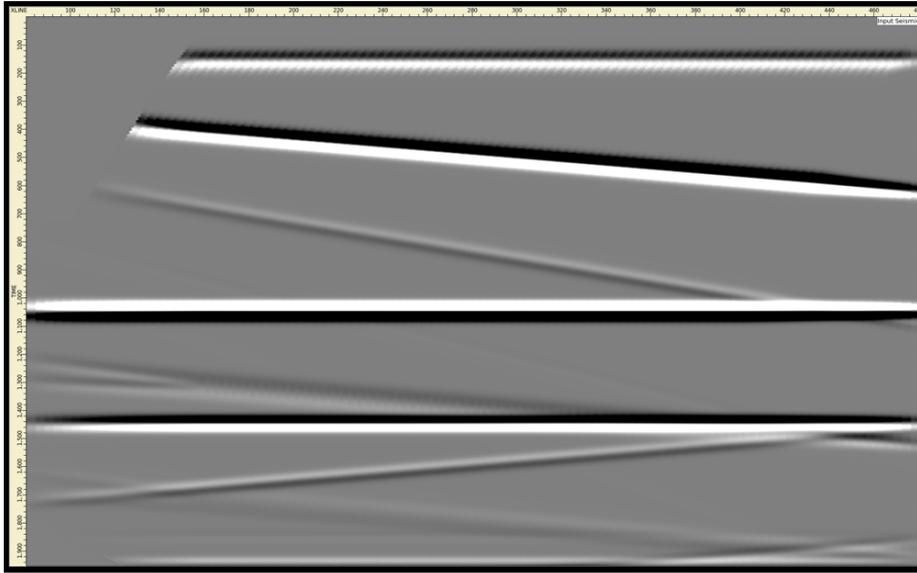
**Figure 4-2:** Synthetic data containing primaries and multiples.
