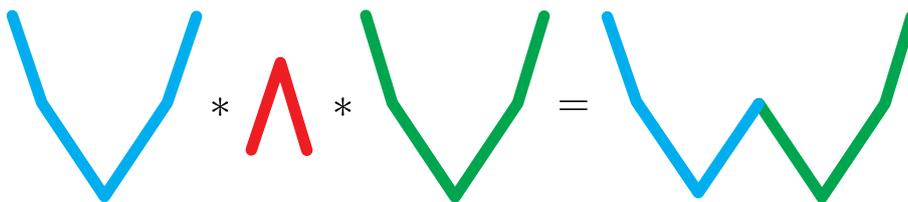
**Figure 3-12:** Illustration how the individual ray-paths are convolved with each other in order to retrieve the multiple ray-path.
