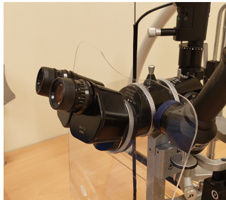
Figure 3 4: Slit lamp without corner piece (left) & with corner piece (right). The corner changes the direction of the eyepiece from horizontal to slightly upwards
