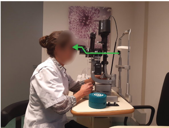
Figure 4 3: Path of the light/image redirected by mirrors inside a Slit Lamp (the green arrow)
