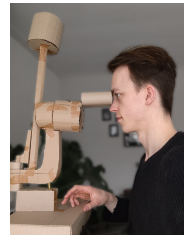
Figure 4.9: Lo-Fi Prototype of a slit lamp, made to understand the effect of different design ideas on the user's posture
