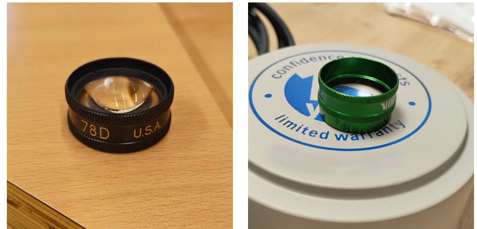
Figure 110: Retinal lenses. A separate lens that is held up between the slit lamp and patient's eye by the ophthalmologist to change magnification, so the doctor can examine the retina. This is called a retinal exam.
