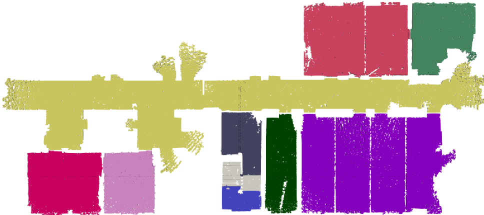
(b) Walkable voxels of floor 2 classified into different rooms, indicated with colours
