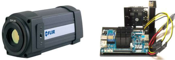
Fig. 1. FLIR SC305 infrared camera (left picture), Pine RockPro 64 (SBC) (right picture).
