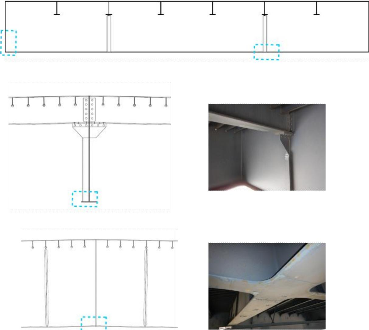
Figure 39 - Critical details of main stringer.
