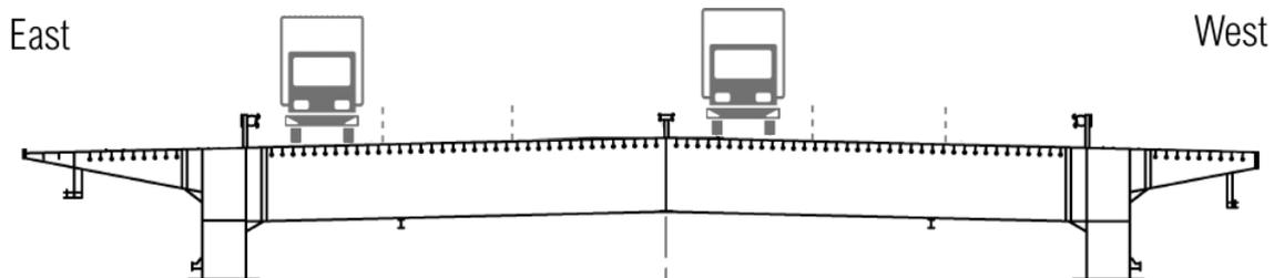
Figure 25. Two separated sections on the eastern Van Brienoord bridge, each with a slow lane [52].
