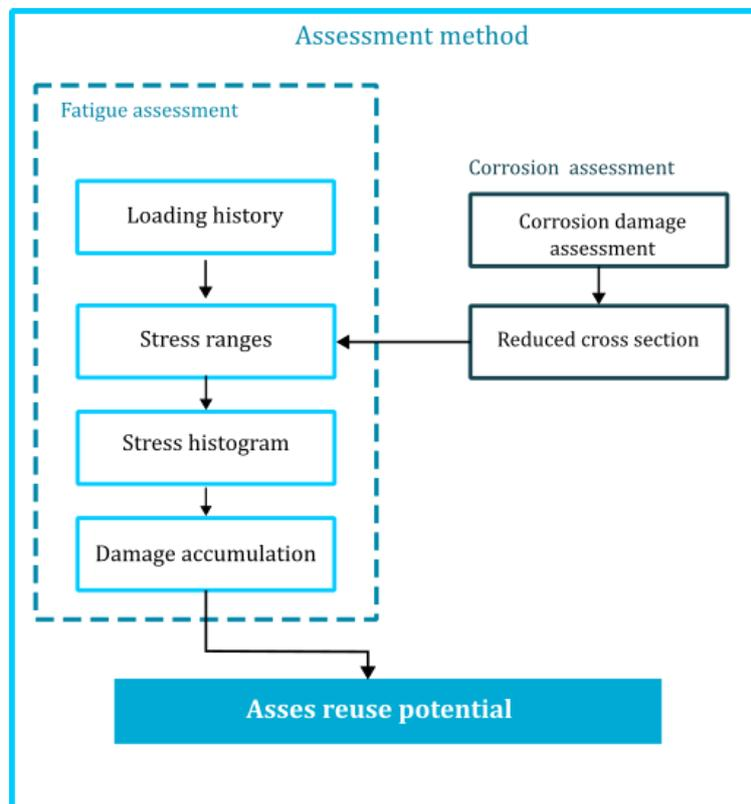
Figure 59 - Flowchart of assessment method used in this study.
