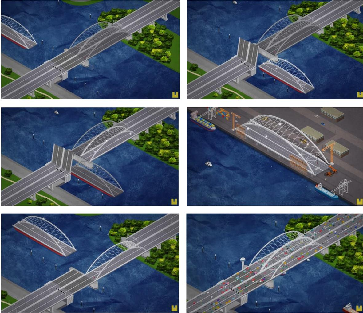
Figure 21. Schematic overview of the renovation of the Van Brienoord bridge [51].
