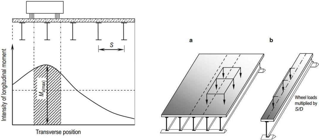
Figure 15 – Concept of load distribution factor and transverse influence line.
