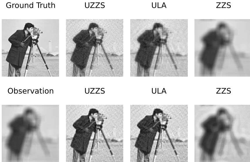
Figure 4.9: Results for the reconstruction of full 256 \times 256 pixels cameraman image using a TV prior. The observed image is obtained with a blur length of 25 pixels and then adding Gaussian noise with standard deviation \sigma = 0.0021 . The reconstructions show the estimated mean after 2 \times 10^3 iterations ( top row ) and after 2 \times 10^5 iterations ( bottom row ) of the samplers based on the states at iterations n \times 10^3 for n = 0, \dots, 200 . The step size for ULA is 1.98/L , for ZZS is 1000/L , where L \approx 518349.52 .
