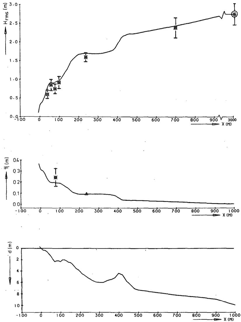
Fig. 2 Comparison of computed results with field data (Egmond beach). For legend, see Figure 1. The vertical line segments indicate one standard deviation on either side of the plotted data point (after Battjes and Stive, 1985)
