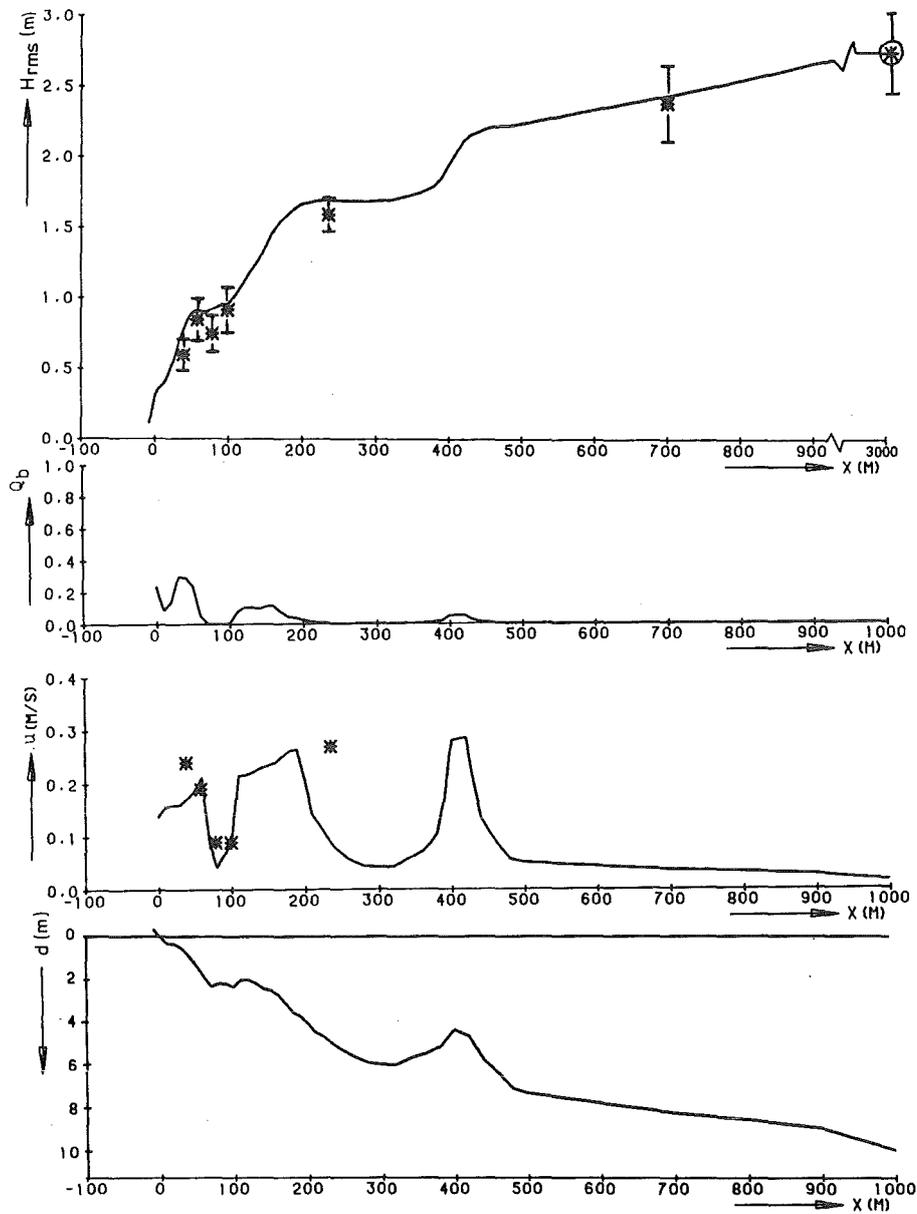
Fig. 5 Results for the same case as shown in Figure 2 (field, Egmond beach). For legend upper and lower diagram see Figure 1. The center diagrams give the fraction of breaking waves ( $Q_b$ ) and the near-bottom return flow velocity ( $u$ ).
