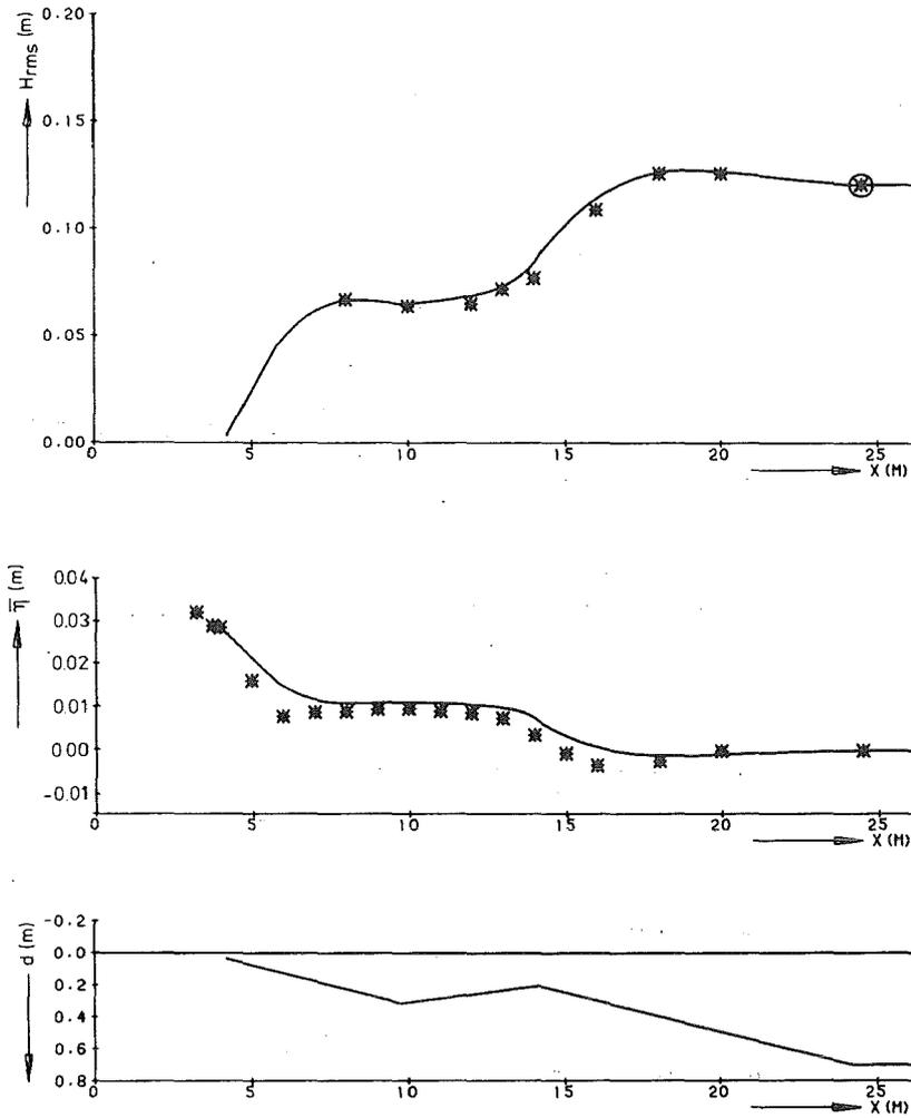
Fig. 1 Comparison of computed results with laboratory data. The figures show profile of bottom elevation below SWL, ( $d$ ), mean water level above SWL, ( $\bar{\eta}$ ), and rms wave height ( $H_{rms}$ ) versus distance normal to shore ( $x$ ). Data points: measured values with offshore reference value encircled. Solid curves: computed values of  $\bar{\eta}$  and  $H_{rms}$  based on a parameterization of  $\gamma$  (after Battjes and Stive, 1985)
