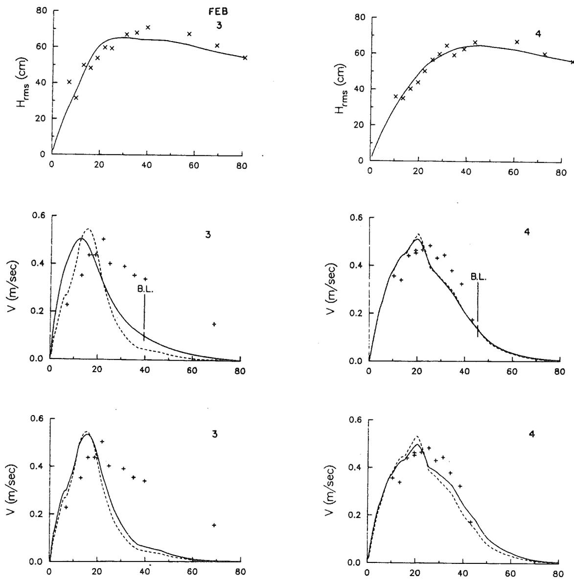
Fig. 3 Upper: rms wave height ( $H_{rms}$ ) versus distance normal to shore; computations (solid lines) and measurements (data points)
