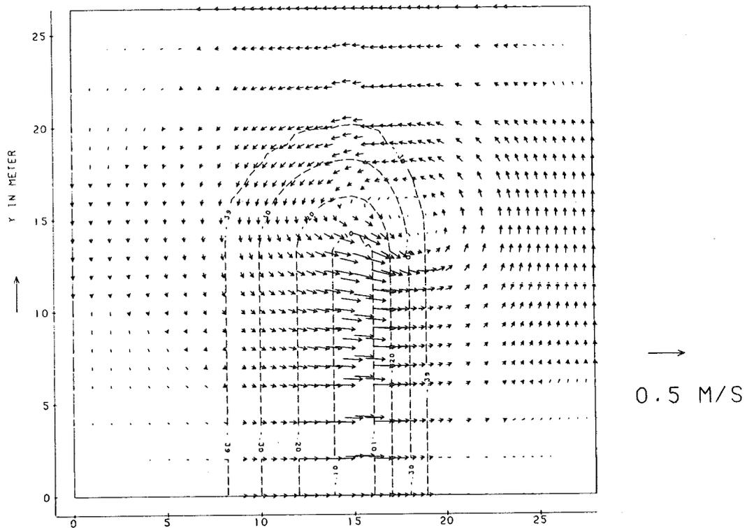
note: The incident wave direction is the positive x-direction; depth contours are in metres; incident significant wave height is 10 cm.
