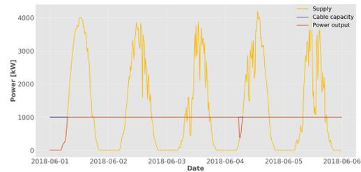
**(b)** LFP Li-ion BESS. Power output over time. Supply of the PV park, in yellow, Cable capacity, in blue and the Power output to the grid, in red, in kW.
