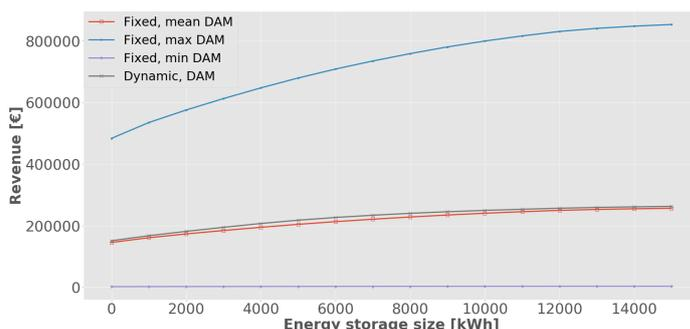
**Figure 42:** Revenue, as a function of the ESS size. The top line is the revenue with a fixed electricity price, maximum DAM price. Bottom line fixed minimum DAM price. The middle two the fixed mean DAM price and a dynamic DAM price.
