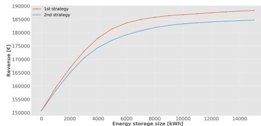
(b) Revenue of a year as a function of the ESS size. 1<sup>st</sup> in red and 2<sup>nd</sup> in blue.
