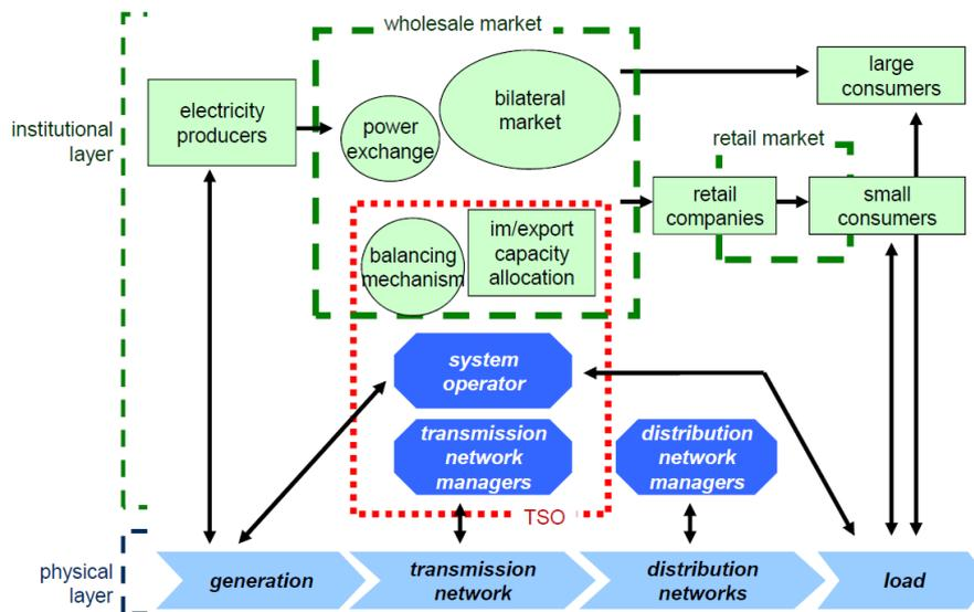
**Figure 5:** Schematic of the Dutch electricity system. Arrows with only one arrow head indicate the electricity trade direction. Double pointed arrows illustrate which institutional actor controls which part the physical layer. [17]
