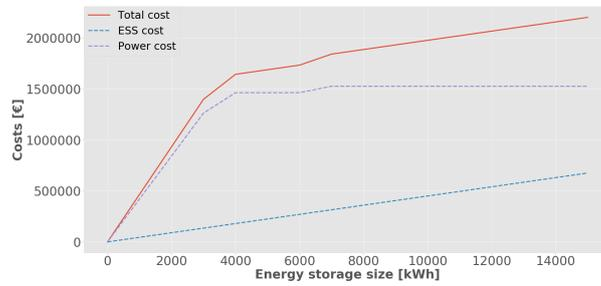
**Figure 31:** Case 1. Total system costs with power system and storage system costs, as a function of the ESS size.
