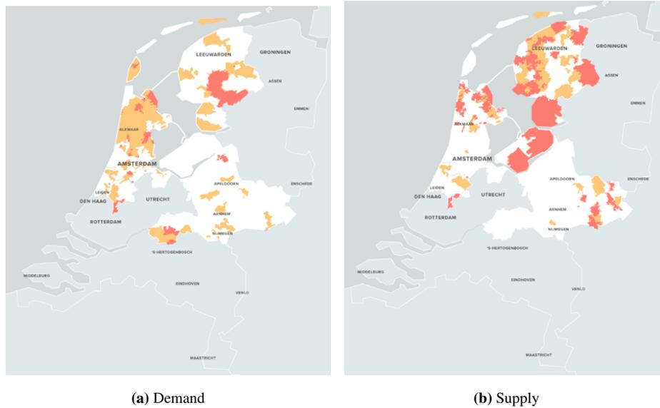
**Figure 3:** Electric transport capacity availability on the distribution network of Liander for installation of extra capacity. For both more demand and more supply. Orange is limited availability, red is no availability. [20]
