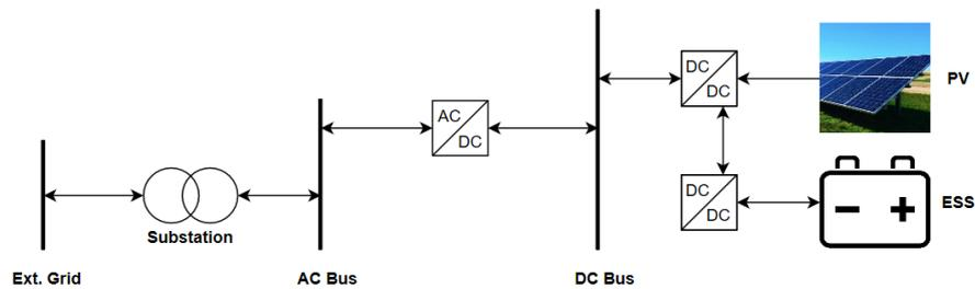
**Figure 15:** Simplified electricity circuit: option 2
