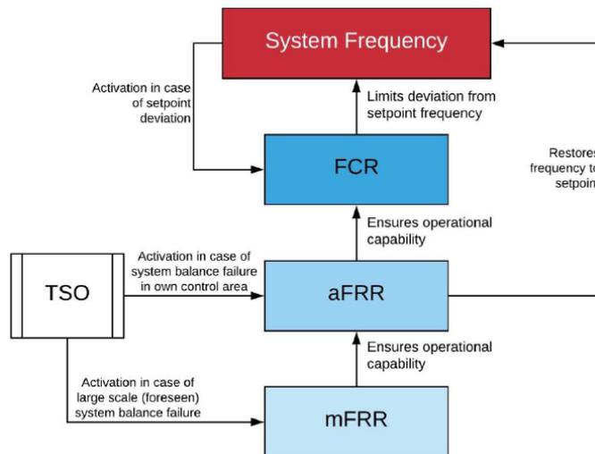
Figure 8: Frequency balancing mechanism schematic [5], based on [6]
