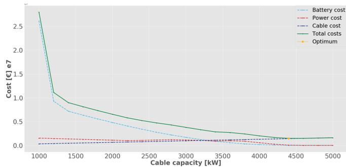
(b) LFP Li-ion BESS. System costs as a function of the cable capacity.
