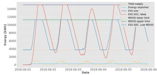
(b) State of charge over time. Showing the electricity supply, yellow, and output, light blue, and ESS size (15 MWh), dark blue, all in kWh. State of charge of the ideal system in red and the SOC of the ESS with low MDOD in light blue. Also the upper and lower SOC limits are plotted
