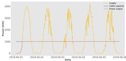
**(a)** Ideal ESS. Power output over time. Supply of the PV park, in yellow, Cable capacity, in blue and the Power output to the grid, in red, in kW.
