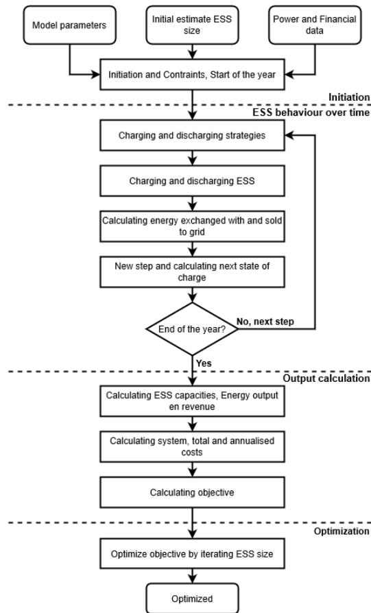
Figure 17: Analytical flowchart of the simulation model, simplified
