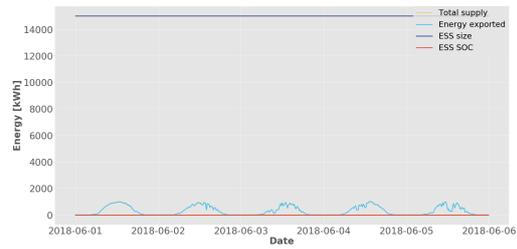
(b) State of charge over time. Showing the electricity supply, yellow, and output, light blue, ESS size (15 MWh), dark blue, and State of charge in red, all in kWh.
