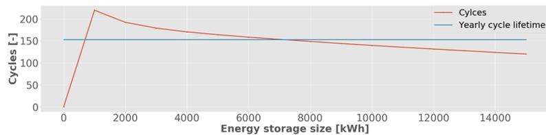
(a) Lead-acid battery, number of cycles and yearly cycle lifetime as a function of the ESS size.
