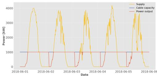
**(c)** Lead-acid BESS. Power output over time. Supply of the PV park, in yellow, Cable capacity, in blue and the Power output to the grid, in red, in kW.
