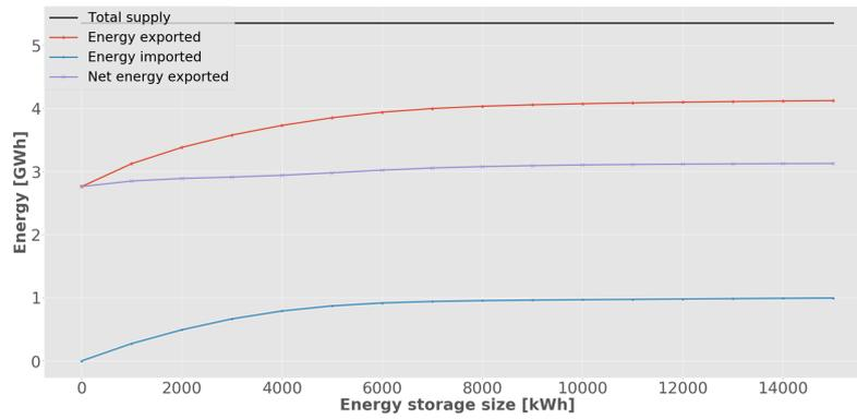
**Figure 61:** Total energy supplied, exported and imported as a function of the ESS size. Results of the 5 MWp PV solar park, cable capacity of 1 MW and Ideal ESS. In black the total amount of energy supplied to the system. In red, marked with stars, is the amount exported to the grid. In blue, marked with dots, is the amount imported from the grid. In blue, marked with x, is the net energy exported.
