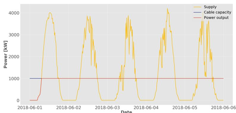
**Figure 27:** Case 1 power output. Supply of the PV park, in yellow, Cable capacity, in blue and the Power output to the grid, in red, in kW over time, five days in June.
