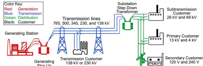
**Figure 1:** Simplified electricity grid with centralized generation and distribution [2]
