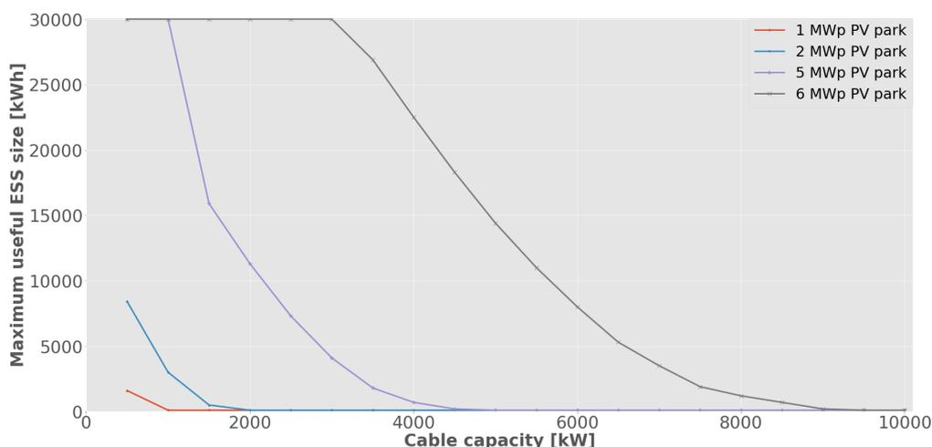
**Figure 60:** Maximum useful Ideal ESS size given the generation and cable capacity.
