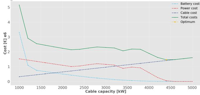
(a) Ideal ESS. System costs as a function of the cable capacity.
