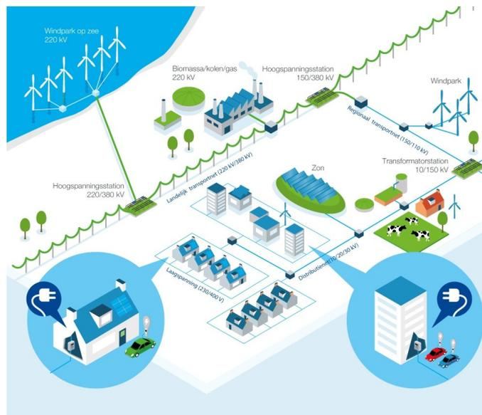
**Figure 2:** Depiction of an electricity grid in the energy transition with centralized and decentralized energy generation [3]
