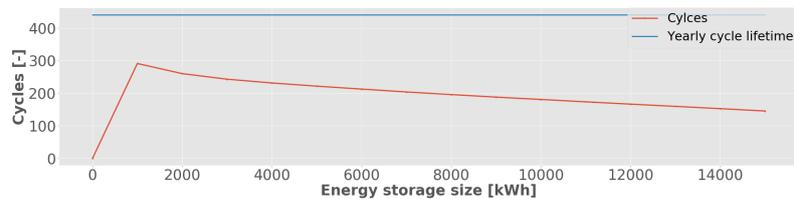
(c) LFP Li-ion battery, number of cycles and yearly cycle lifetime as a function of the ESS size.
