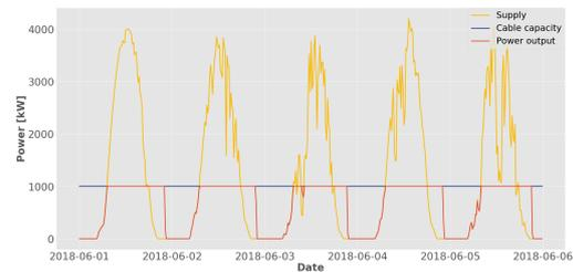
**(d)** Flywheel ESS. Power output over time. Supply of the PV park, in yellow, Cable capacity, in blue and the Power output to the grid, in red, in kW.
