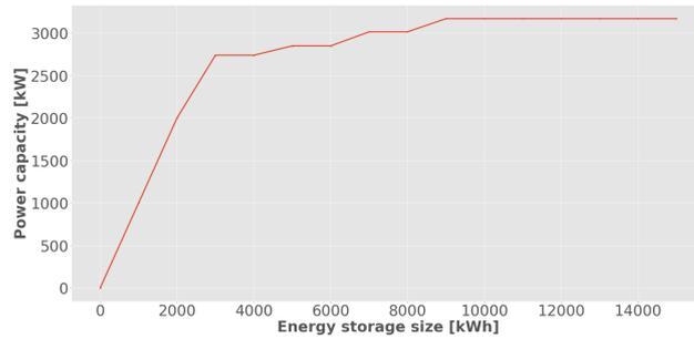
(a) Power capacity, as a function of the ESS size.
