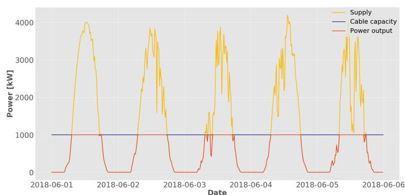
**Figure 26:** Base case power output. Supply of the PV park, in yellow, Cable capacity, in blue and the Power output to the grid in kW, in red.
