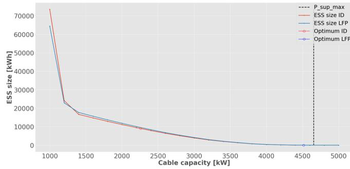
(a) Storage size [kWh] as a function of the cable capacity.
