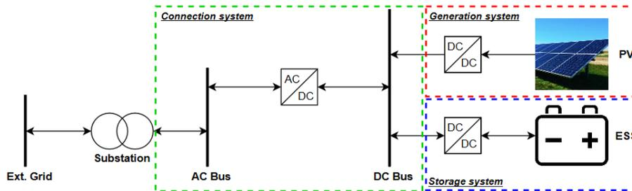
**Figure 24:** Electricity system schematic with system boundaries. Red generation system, blue ESS system and green connection system.
