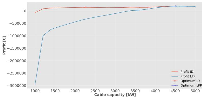
**Figure 58:** Profit as a function of the cable capacity. A comparison between a system with an Ideal ESS and a LFP BESS.
