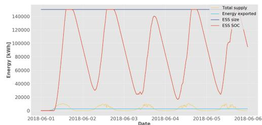
(b) State of charge over time. Showing the electricity supply, yellow, and output, light blue, and ESS size (150 MWh), dark blue, and state of charge, red, in kWh.
