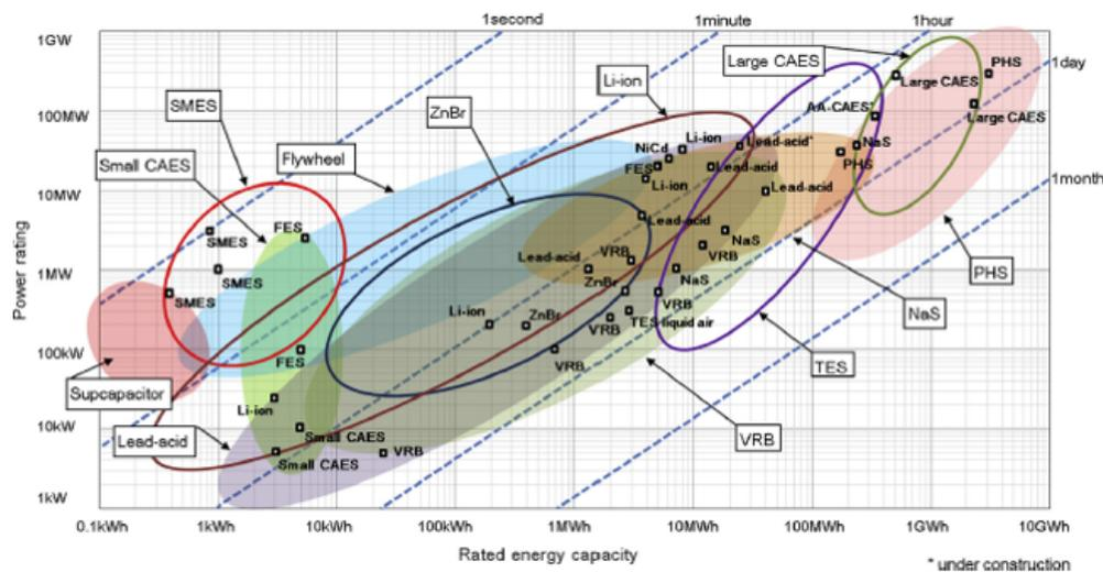
**Figure 11:** Energy storage systems compared at rated energy capacity vs power rating [7].
