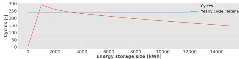
(b) NMC Li-ion battery, number of cycles and yearly cycle lifetime as a function of the ESS size.
