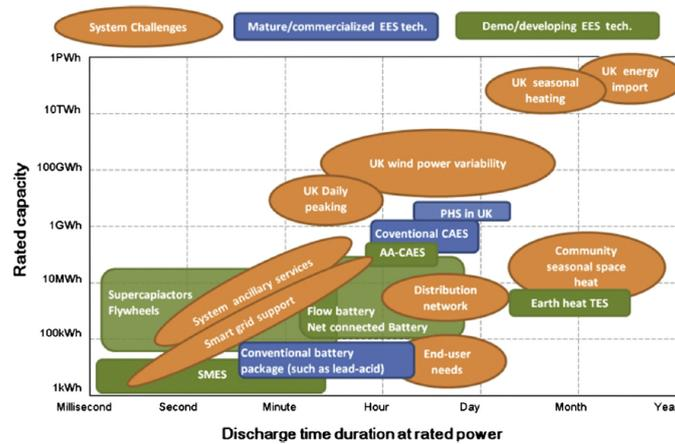
**Figure 12:** Electrical energy storage systems and system challenges, Discharge time vs rated capacity [7].
