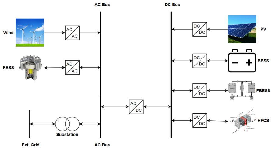
**Figure 13:** Electric circuit of a hybrid system with a PV solar- and wind park and different storage technologies [45].
