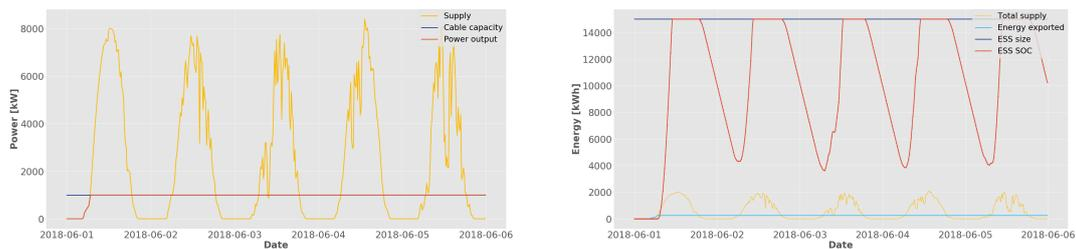
(a) Power output over time. Supply of the PV park, in yellow, Cable capacity, in blue and the Power output to the grid, in red, in kW.
