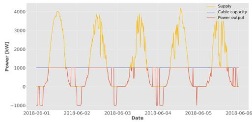
(a) Power output over time. Supply of the PV park, in yellow, Cable capacity, in blue, and the Power output to the grid, in red, in kW. Positive for export and negative for import.
