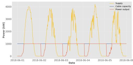
(a) Power output over time. Supply of the PV park, in yellow, Cable capacity, in blue and the Power output to the grid, in red, in kW.
