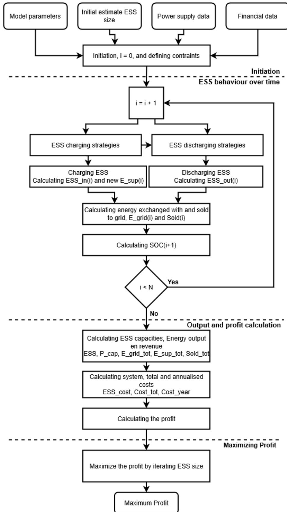
Figure 25: Analytical flowchart of the simulation model
