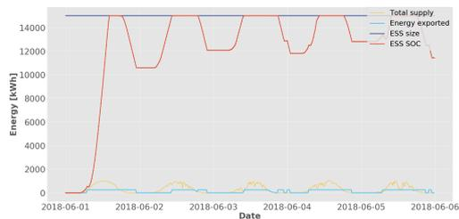
**(b)** State of charge over time. Showing the electricity supply, yellow, and output, light blue, and ESS size (15 MWh), dark blue, and state of charge, red, in kWh.
