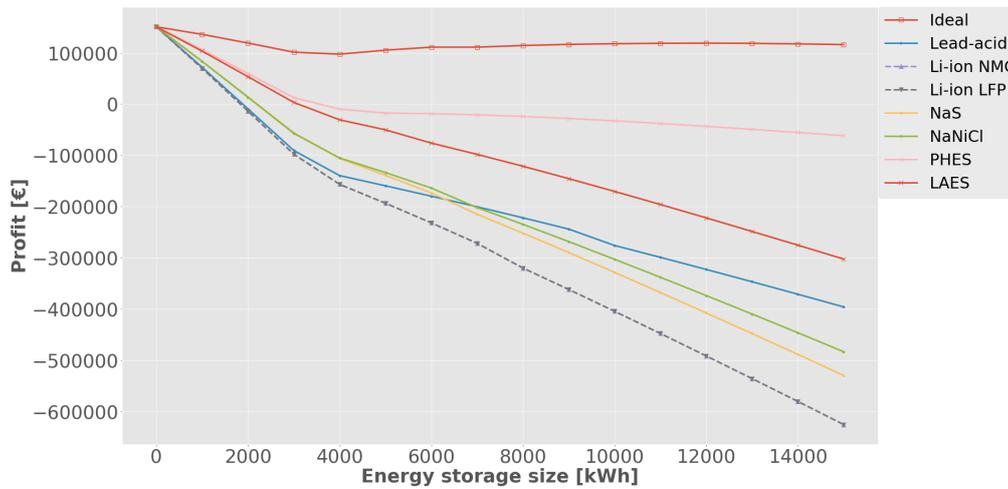
**Figure 52:** Profit as a function of the ESS size. A comparison of all technologies, except for VRB, ZnBr, FES and HFCS.
