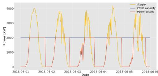
(a) Power output over time. Supply of the PV park, in yellow, Cable capacity, in blue and the Power output to the grid, in red, in kW.
