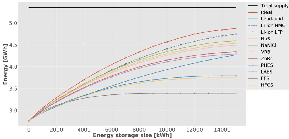
**Figure 51:** Energy output as a function of the ESS size. A comparison of all technologies.
