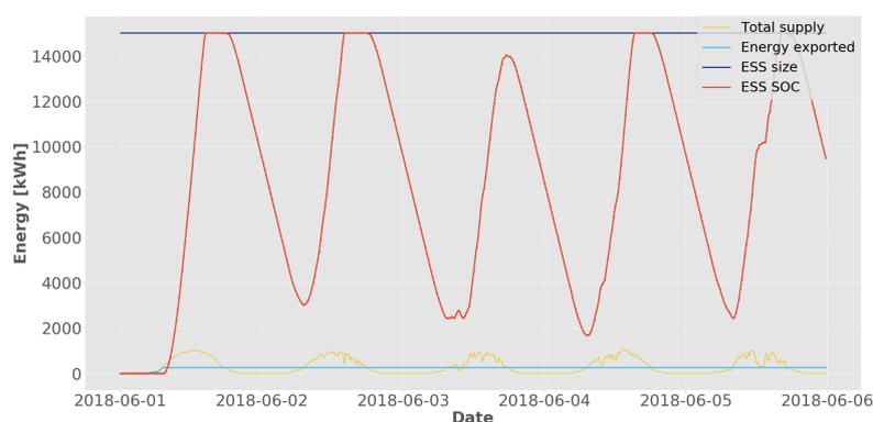
**Figure 28:** Case 1. Showing the electricity supply, yellow, and output, light blue, and ESS size (15 MWh), dark blue, and state of charge, red, in kWh over time, five days in June.
