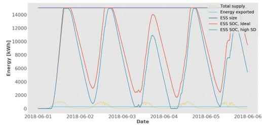
(b) State of charge over time. Showing the electricity supply, yellow, and output, light blue, and ESS size (15 MWh), dark blue, all in kWh. State of charge of the ideal system in red and the SOC of the ESS with high self-discharge in light blue.
