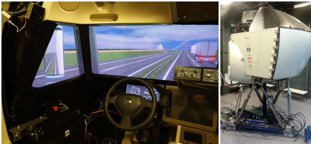
Figure 1. The truck driving simulator. Left = cabin view; Right = outside view
