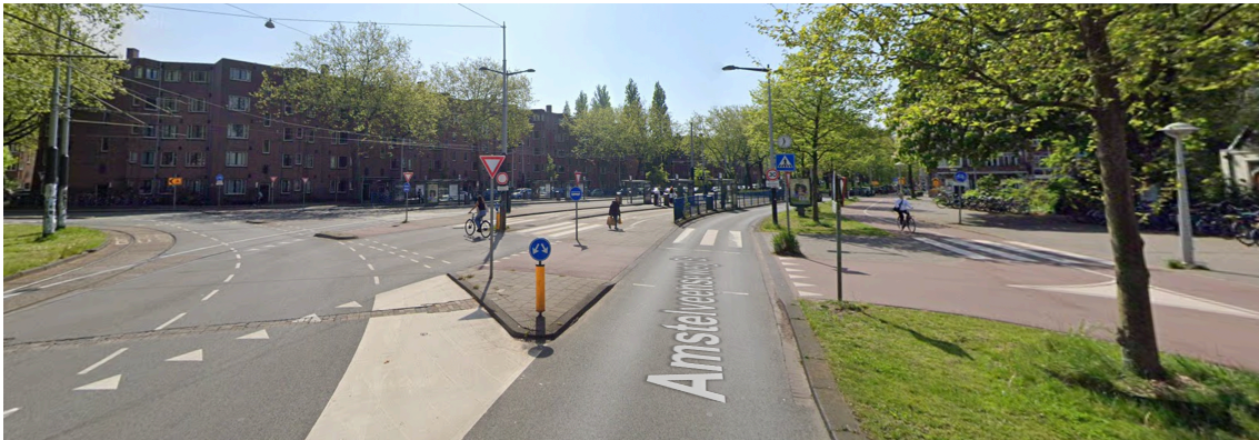
(c) Haarlemmermeerstationplein, from the perspective of the motor vehicle, looking south to exit with the two south-bound bus stops in the center of the image. Note that this vehicular crossing, vehicles have yielding priority (bicycles have to yield to cars).
