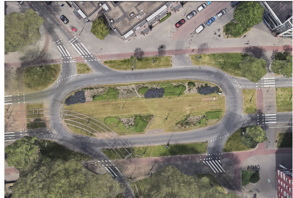
(b) Aerial view of Putsebocht tram stop in Rotterdam, where yielding priority is given to vehicles. In addition, there were some wrong way bicycling observed at the southern and western crossings.
