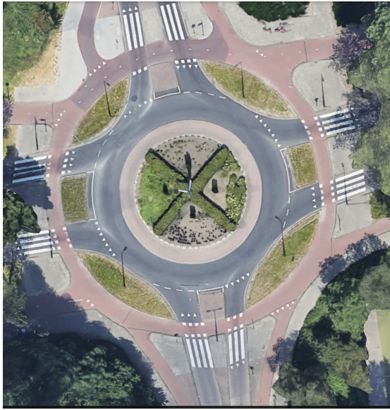
(a) Aerial view of roundabout on Gordelweg, where the Noorderkanaal and A20 highway to the north are the reason for many north/south and southwest corner to northeast corner bicycle movements
