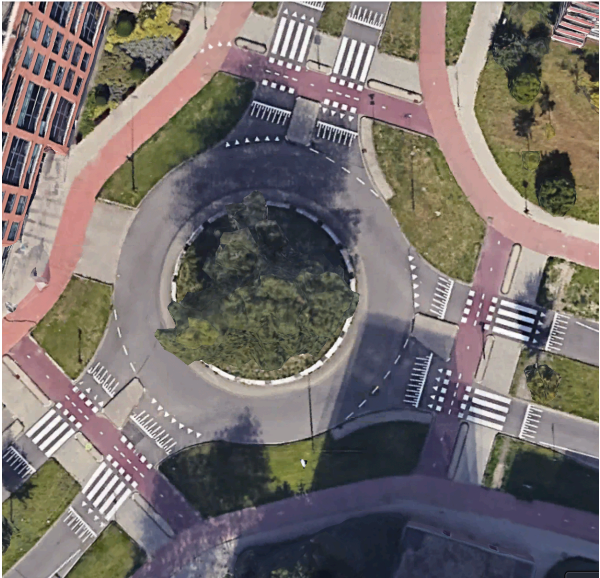
Figure 2.1: Satellite view of Meerzichtlaan, Zoetermeer, where the two-way bicycle facility is clearly present from the pavement markings. Note how the bicycle facilities have a bent shape that provides more buffer width between the bicycle facility and the vehicular lanes. The grey pavement on the left side of the roundabout is a driveway and not a road. Image courtesy of Google Earth
