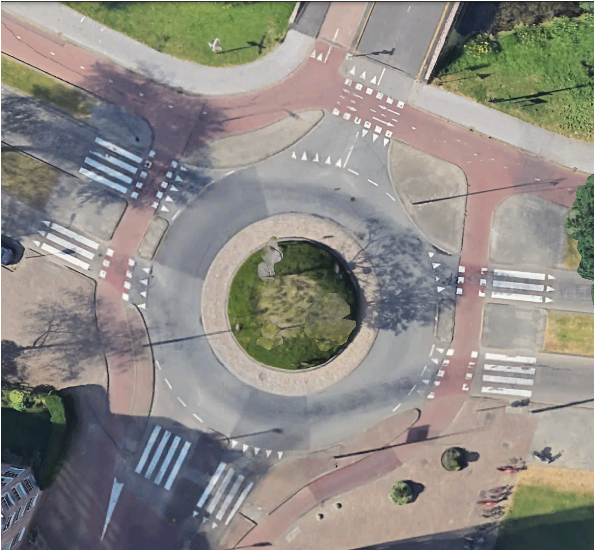
Figure 2.2: Satellite view of Kralingseweg and Plaszoom intersection, Rotterdam. The notable features of this roundabout are that there is no bicycle crossing on the south side or a bicycle path on the south side of the Kralingseweg approaching the roundabout on either side (the two-way bicycle path on the north side serves both directions). Attention is due at the shape of the bicycle facility around this roundabout, as one can see the bent path shape clearly in the NW corner whilst the three other corners resemble the circular shape (closely following the shape of the vehicular lane). Another thing to note is that two-way bicycle facility connection on the NE corner which is the main bicycle path crossing Kralingse Bos. Image courtesy of Google Earth
