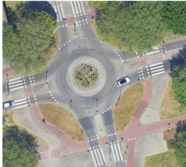
(b) Aerial view of Prinsenlaan roundabout, where bicyclists were observed going the wrong way on the northside of the roundabout to access the apartments located on that side.
