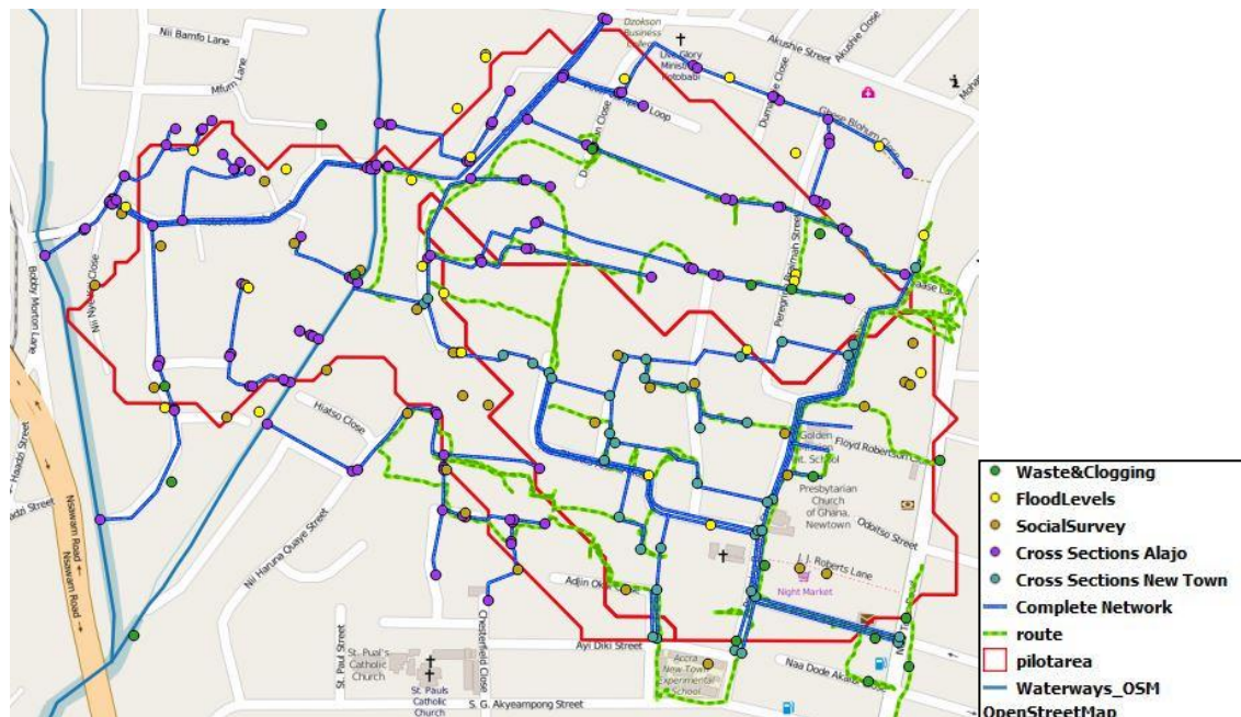
Figure 23 Drainage network constructed in QGIS based on Field Papers, data points and GPS tracks
