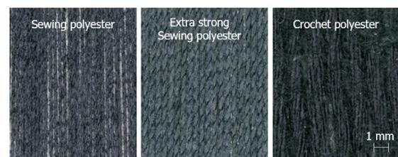
**Fig. 4.** Microscope images of a sewing polyester (‘SP’), extra strong sewing polyester (‘ESSP’) and crochet polyester (‘CP’) spool.
