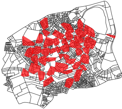
(a) Conflict-based clusters with a high density categorisation at 50 minutes of a simulation with 400 aircraft.
