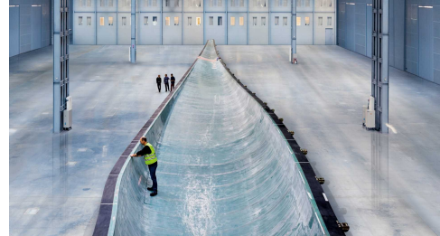
Figure 2.10: Blade mould at the Siemens blade factory in Hull. Retrieved from Manufacturer (2018)
