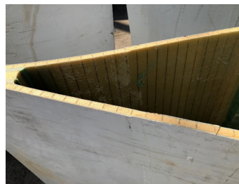
Figure 4.28: Detailed picture of a shell panel. Picture provided by the Re-Wind Network
