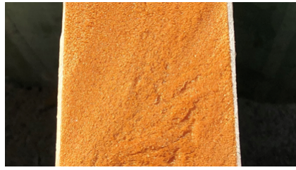
Figure 4.29: Detailed picture of the shear web. Picture provided by the Re-Wind Network
