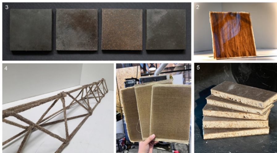
Fig. 1. Overview of PFRP prototypes: 1. Flax-PLA Laminate (Sect. 2.1), 2. Flax Fiber Reinforced Composite (Sect. 2.3), 3. Bio-waste-based composites (Sect. 2.3), 4. Truss-to-GO (Sect. 2.4) and 5. PLAX (Sect. 2.5).
