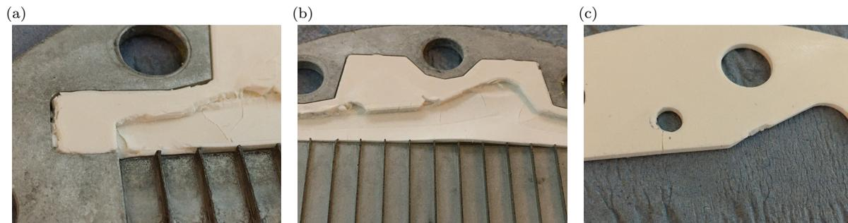
Figure 5.16: The result of chemical and mechanical loading on the insert and spacer. (a) Lamination of the insert, probably as a result of the acidic or alkaline environment. The channel width of this design is 6.2 mm. (b) Deformation of the insert because the fit in the cavity was too tight. (c) A crack in the spacer as a result of mechanical loading.
