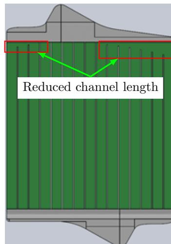
Figure 4.6: A variation to the design with the channels, the channel length is varied over the cell width.
