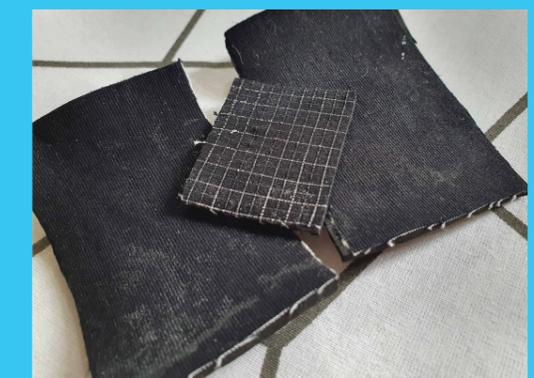
Photo of first neoprene prototypes using Vliesofix
