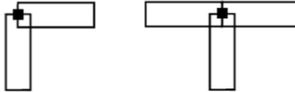
Figure 4-10: Geometrical approximation of nodes and elements at web-flange junctions
