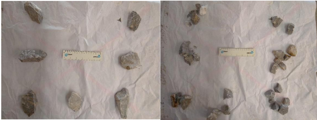
Figure 46 Example of Samples for Point Load Test Prior test and post-testing
