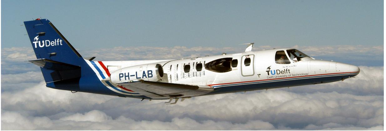
**Fig. 3** The PH-LAB research aircraft operated by Delft University of Technology. The Cessna Citation 550 is a CS-25 certified aircraft.
