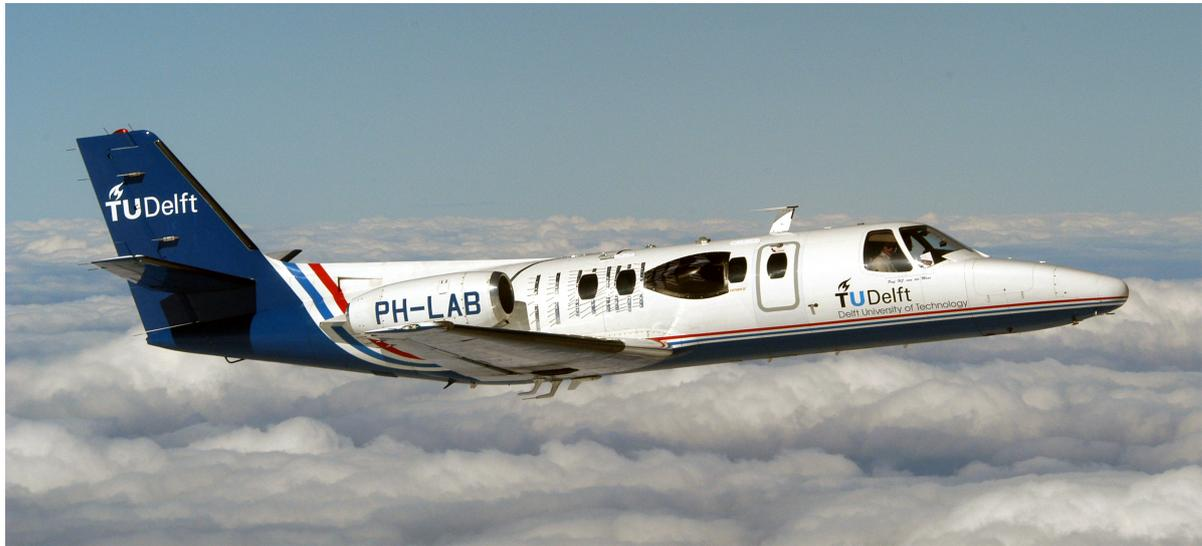
Figure 1.1: The PH-LAB research aircraft operated by Delft University of Technology. The Cessna Citation 550 is a CS-25 certified aircraft with a fly-by-wire control system certified for experimental flight controllers.
