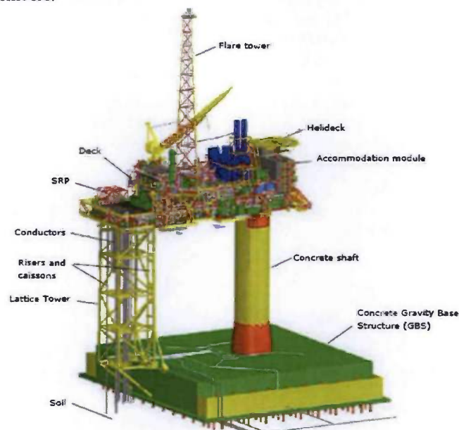
Figure 2 South Arne Platform in the Danish sector at 60 m of water depth
