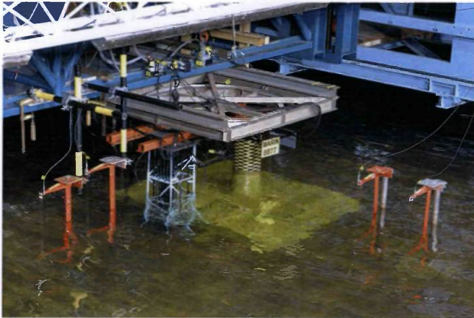
Figure 6 Small scale tests of the GBS and lattice tower combined in the basin
