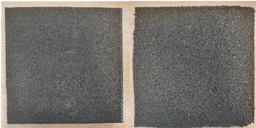
Figure 35: Test 1 – Used standard tile made into a standard tile again
