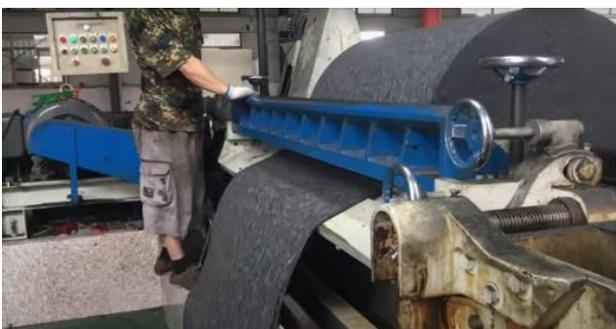
Figure 12: Peeling process of a cold moulded rubber cylinder
