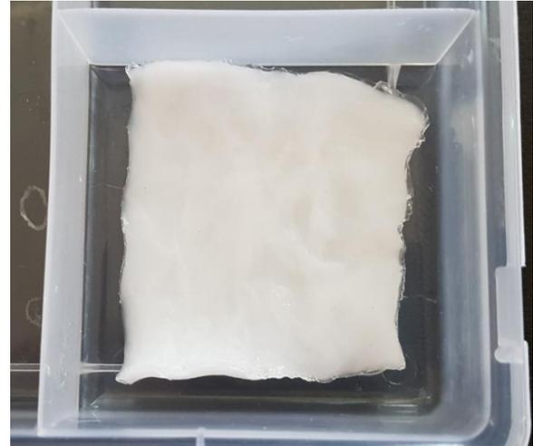
Figure 61 Shrinking of a PVA (7m%) sample after 8 freeze-thaw cycles (8 hours freezing and 8 hours thawing).
