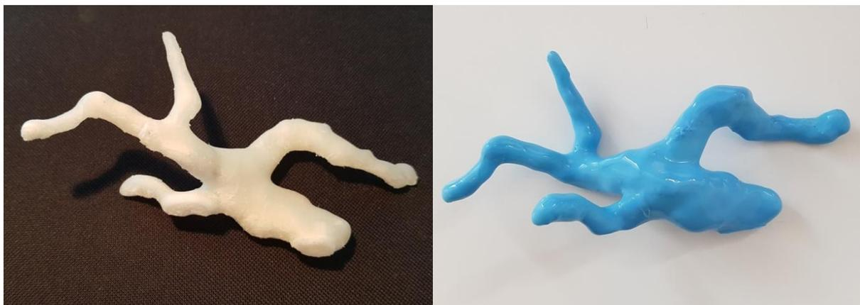
**Figure 38** (Left) 3D-printed structure of the simplified portal vein. (Right) Silicone portal vein with the 3D-printed structure still inside the vein.
