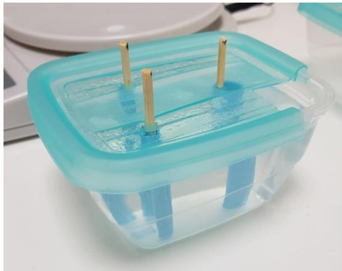
Figure 74 Silicone tubes embedded in liquid PVA, just after it was poured into the container.
