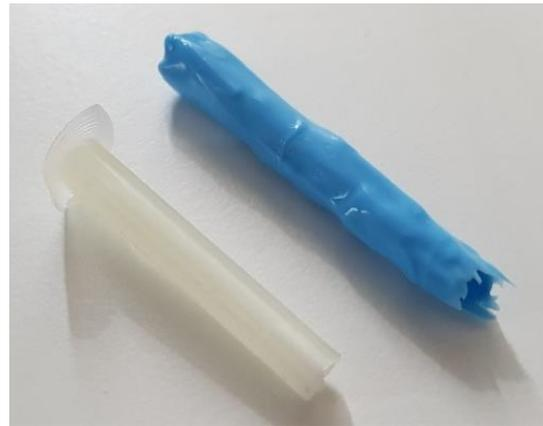
**Figure 37** 3D-printed rod (5 mm diameter) made of water-soluble PVA (white) and a thin-walled silicone tube, created using a rod of water-soluble PVA (blue).
