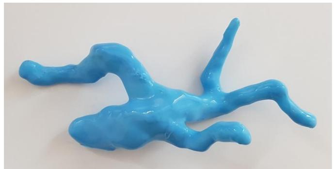
Fig. 7. Silicone blood vessel created with a simplified, 3D-printed, portal vein model.
