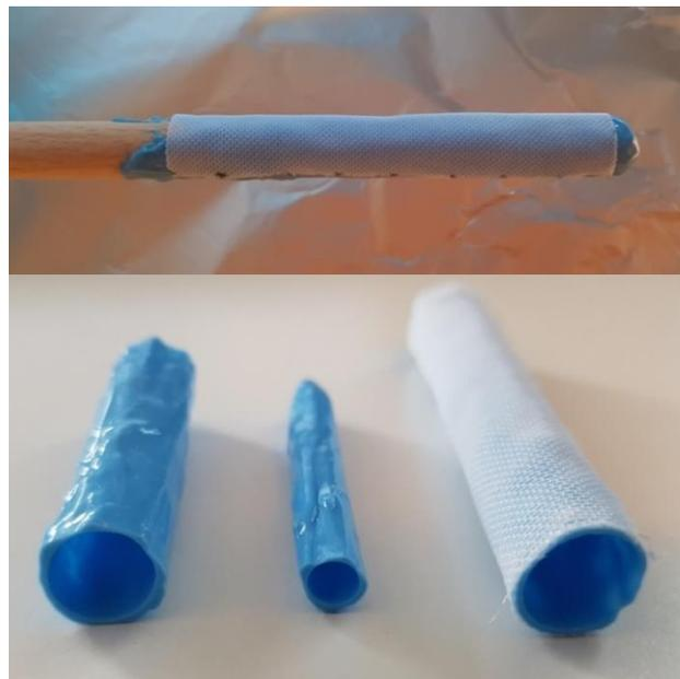
Figure 36 Silicone and mesh fabric on a 10 mm diameter wooden rod (top) and thin-walled silicone tubes with and without mesh fabric (bottom).
