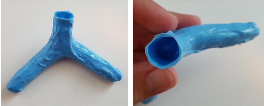
Figure 40 Thin-walled and T-shaped silicone tube, made using a Monster Clay structure.
