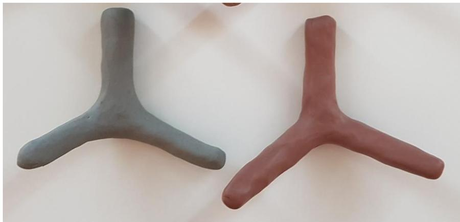
**Figure 39** Two T-shaped samples to mimic a blood vessel structure, made of plasticine (left) and Monster Clay (right). The diameter of both structures is about 10 mm.
