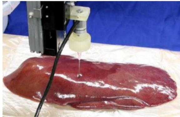
Figure 10 Experimental setup for needle insertions in porcine liver and its blood vessels. Retrieved from [11].
