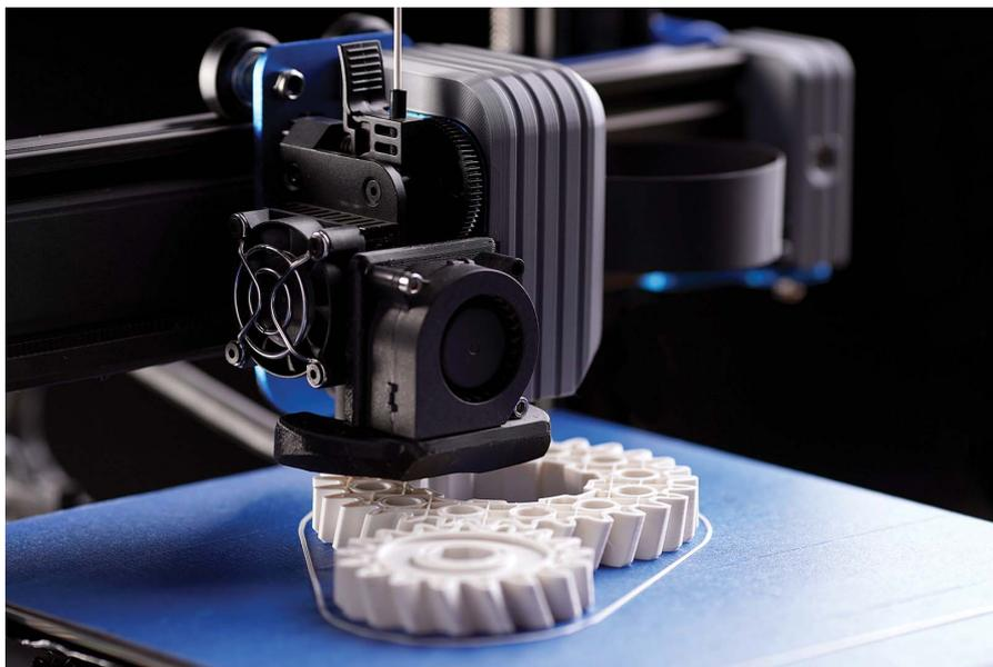
Figure 1.1: Fused Deposition Modeling [20]
