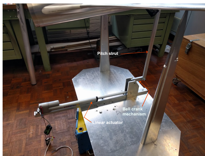
Figure 3.11: Linear actuator and bell crank mechanism setup
