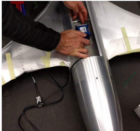
Figure 3.9: Angle of attack sensor mounting in the scaled model
