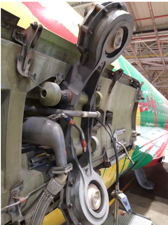
Figure 3.23: Reference dampers used on MD11 - fuselage part.
