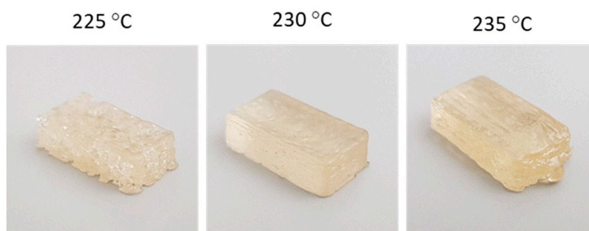
Figure 8. Pictures of the 3D printed SH-TPU samples of approximately 10 × 20 × 5 mm.
