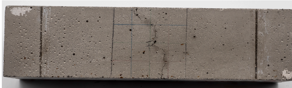
Fig. 11. Macro crack formation in softening stage (valid result).
