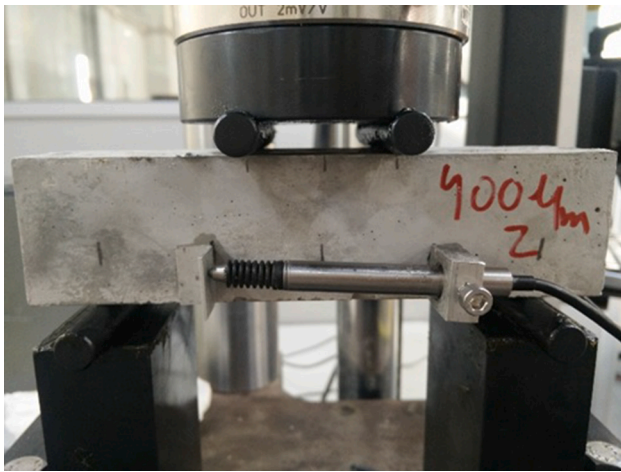
Fig. 1. Four-point bending test.
