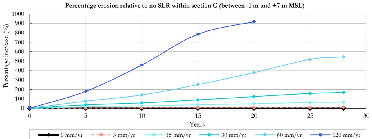
Figure 5-15: Erosion relative to no SLR (%) for increasing SLR rates within the northern section, C (between -1 m and +7 m MSL)
