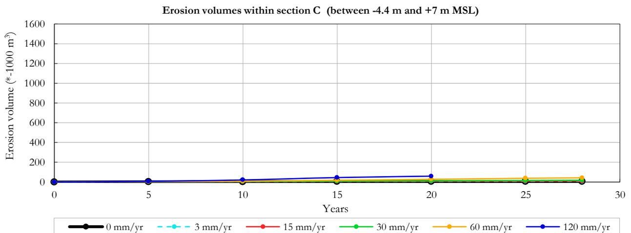
Figure 5-9: Change in erosion volumes over time for increasing SLR rates within the northern section, C (between -4.4 m and +7 m MSL)
