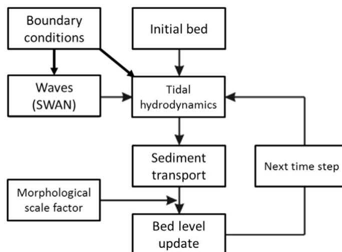
Figure 4-1: Morphodynamic feedback loop applied in Delft3D (Luijendijk et al., 2017)
