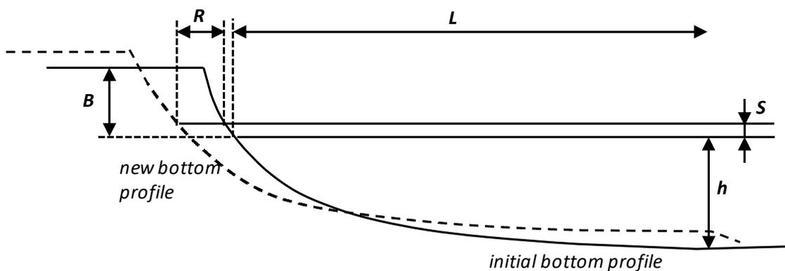
Figure 2-3: Geometric response of nearshore profile to SLR according to Bruun (1962)
