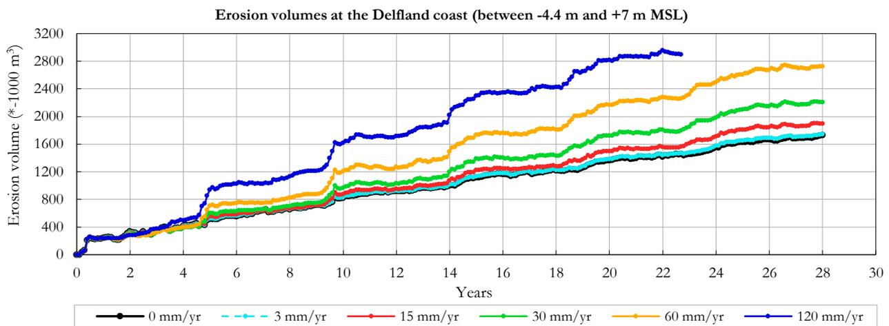
Figure 5-5: Cumulative erosion volumes plotted per timestep for each SLR scenario at the Delfland coast (between -4.4 m and +7 m MSL)
