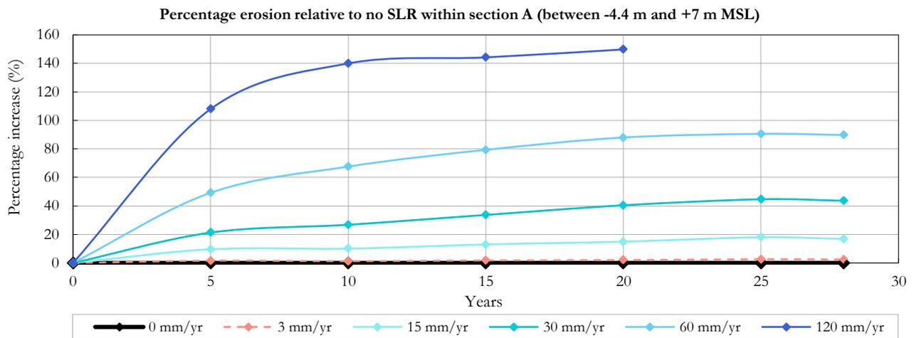
Figure 5-10: Erosion relative to no SLR (%) for increasing SLR rates within the southern section, A (between -4.4 m and +7 m MSL)
