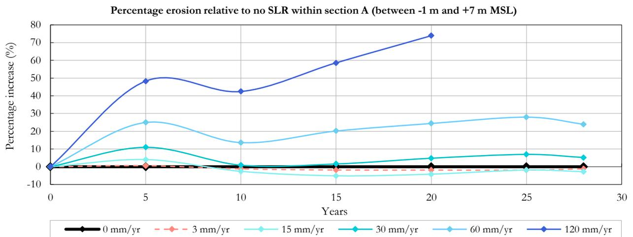
Figure 5-12: Erosion relative to no SLR (%) for increasing SLR rates within the southern section, A (between -1 m and +7 m MSL)
