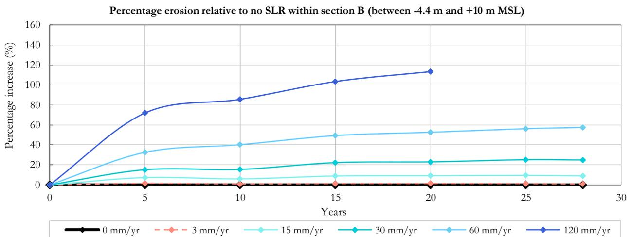
Figure 6-5: Erosion relative to no SLR (%) for increasing SLR rates within the central section, B (between -4.4 m and +10 m MSL)
