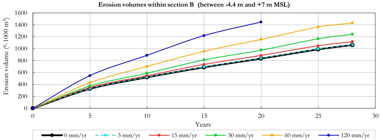
Figure 5-8: Change in erosion volumes over time for increasing SLR rates within the central section, B (between -4.4 m and +7 m MSL)
