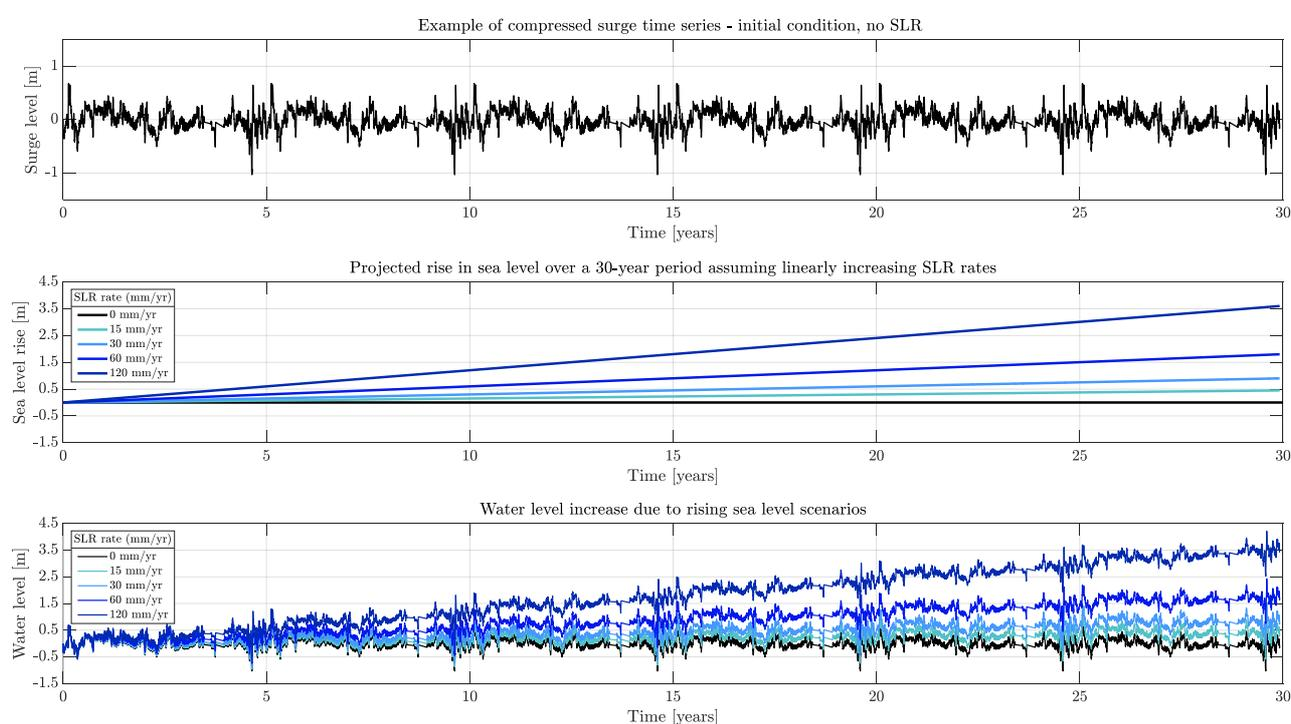
Figure 4-4: Water level adjustment to account for SLR
