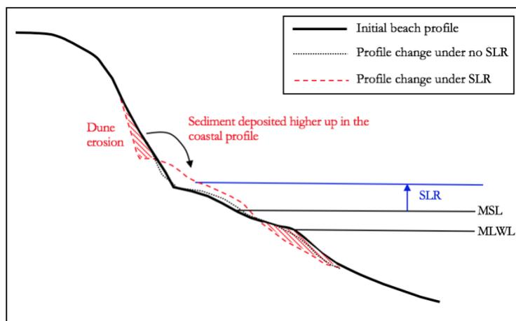
Figure 6-2: Cross-shore erosion and deposition due to SLR
