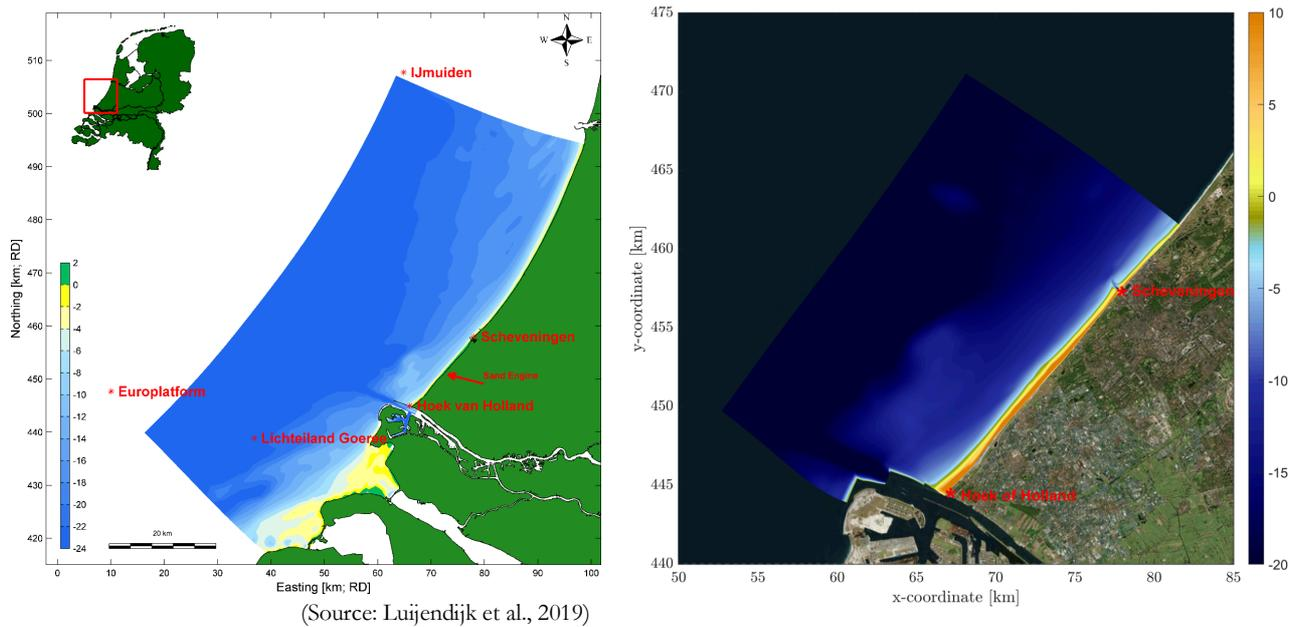
Figure 4-2: Geographical setting of the Delfland coast and larger-scale wave model domain in calibrated model (left). Model domain with initial bed elevations in meters (right).
