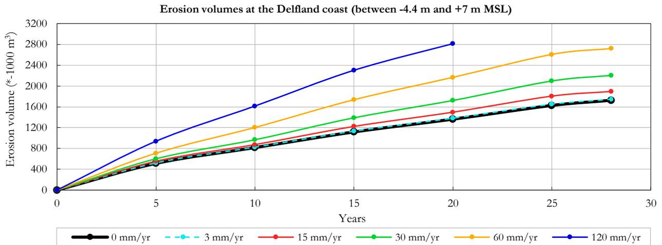
Figure 5-6: Change in erosion volumes over time for increasing SLR rates at the Delfland coast (between -4.4 m and +7 m MSL)
