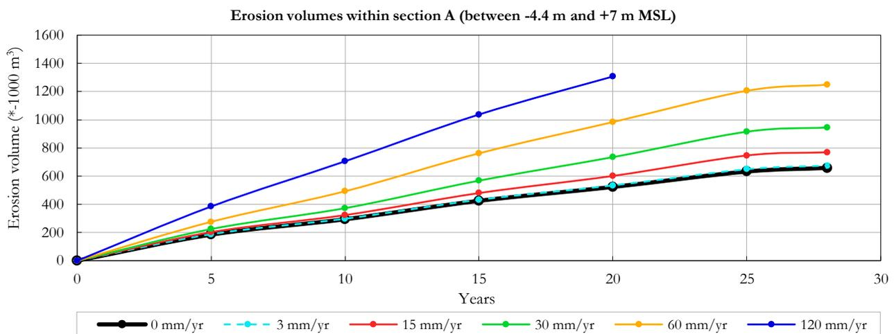
Figure 5-7: Change in erosion volumes over time for increasing SLR rates within the southern section, A (between -4.4 m and +7 m MSL)
