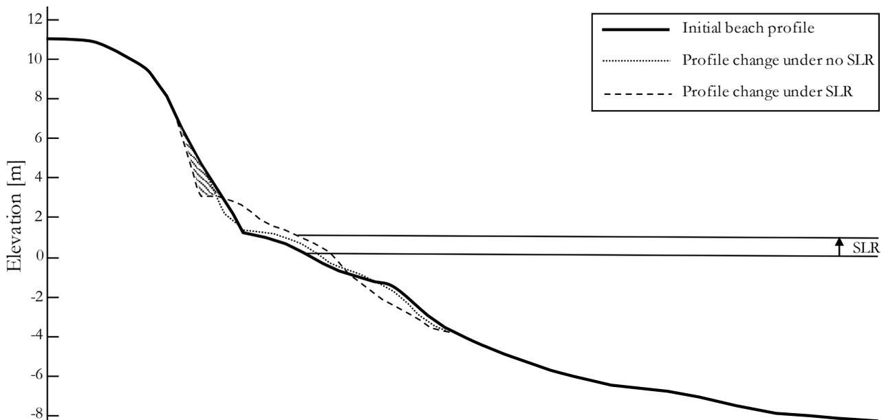
Figure 5-3: Schematic diagram showing beach profile changes and additional erosion due to SLR
