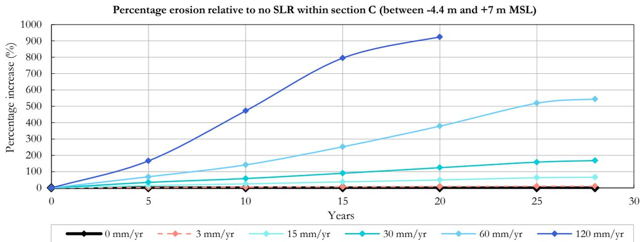
Figure 5-14: Erosion relative to no SLR (%) for increasing SLR rates within the northern section, C (between -4.4 m and +7 m MSL)
