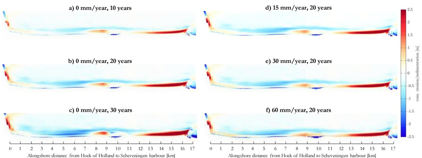
Figure 5-1: Computed bed level changes: no SLR scenario over time (left), increasing SLR rates at the 20-year time interval (right).
