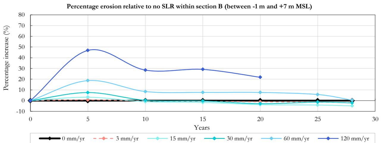
Figure 5-13: Erosion relative to no SLR (%) for increasing SLR rates within the central section, B (between -1 m and +7 m MSL)
