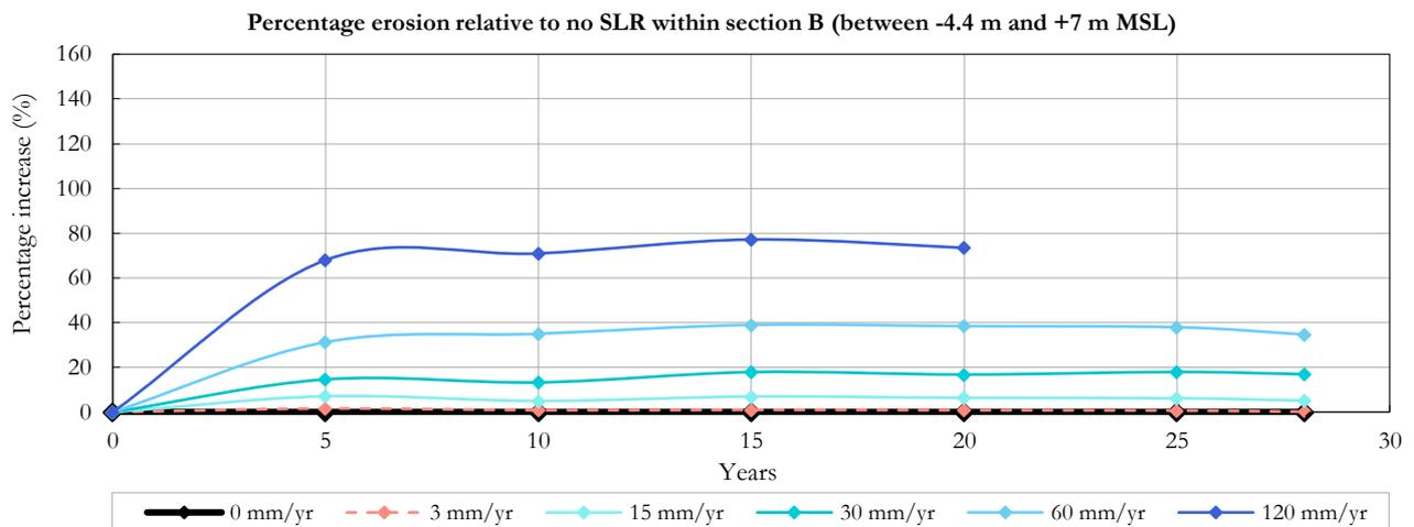
Figure 5-11: Erosion relative to no SLR (%) for increasing SLR rates within the central section, B (between -4.4 m and +7 m MSL)
