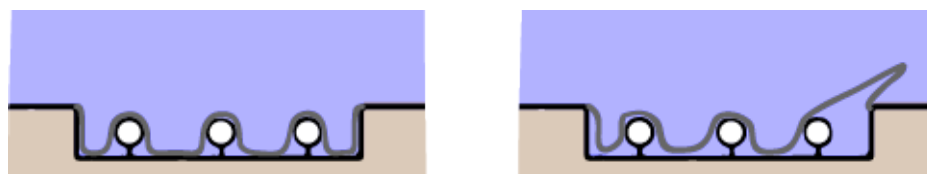
Figure 9.12: Impression of failed storing of the membrane, the left picture shows a correctly stored membrane and the right one shows a fold
