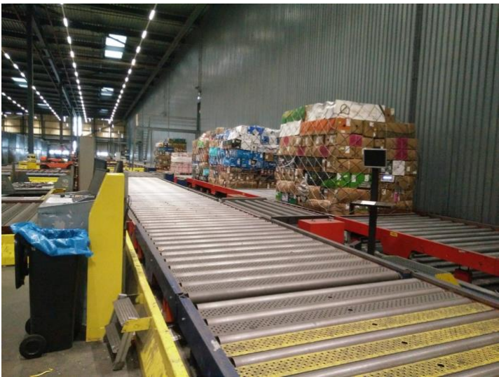
Figure 18. Freight belt directly connects airside with landside
