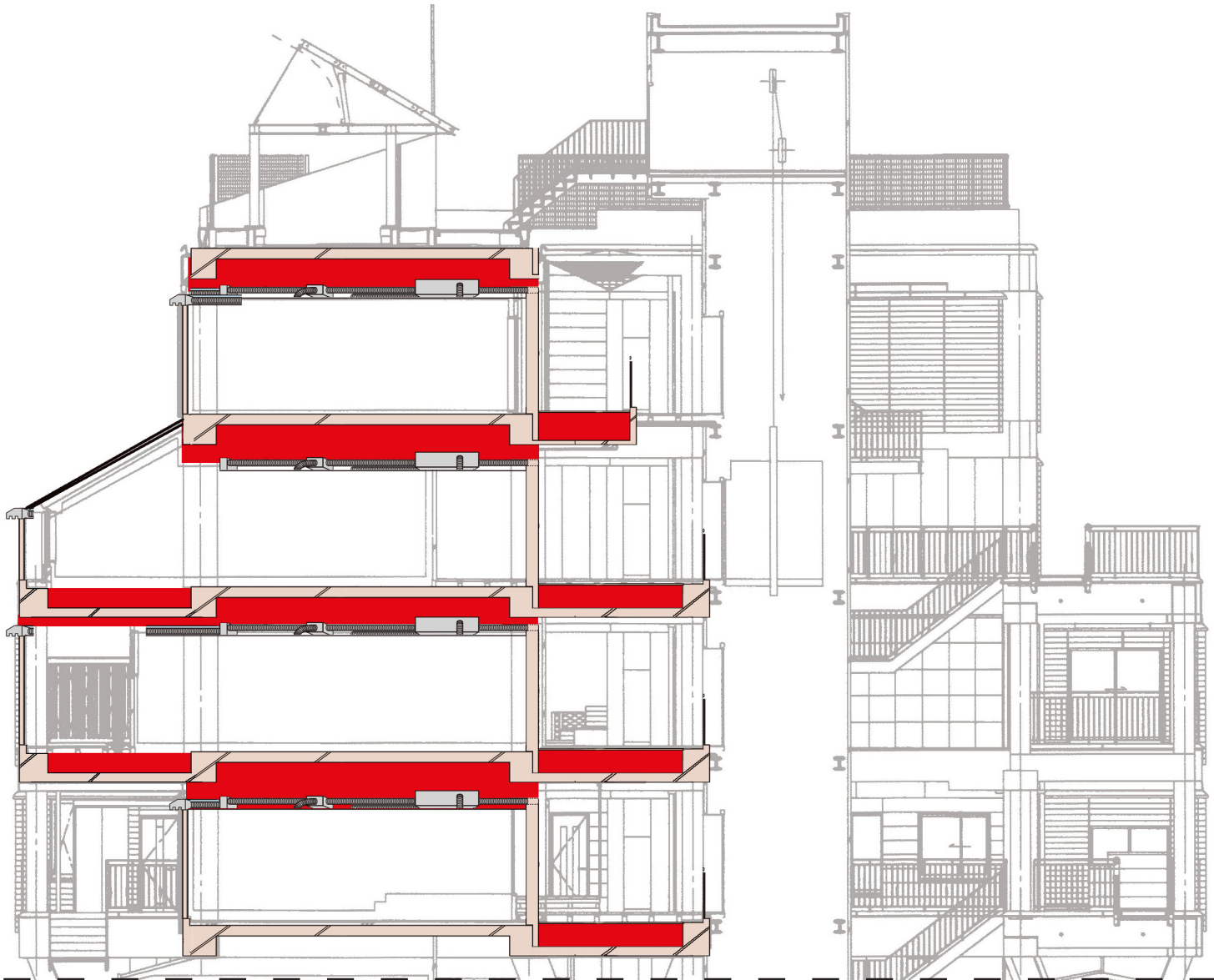
Figure 86. Horizontal Service Infrastructure distribution, highlighted in red (Support) (Source: Osaka Gas Co, 2015; modified by author)
