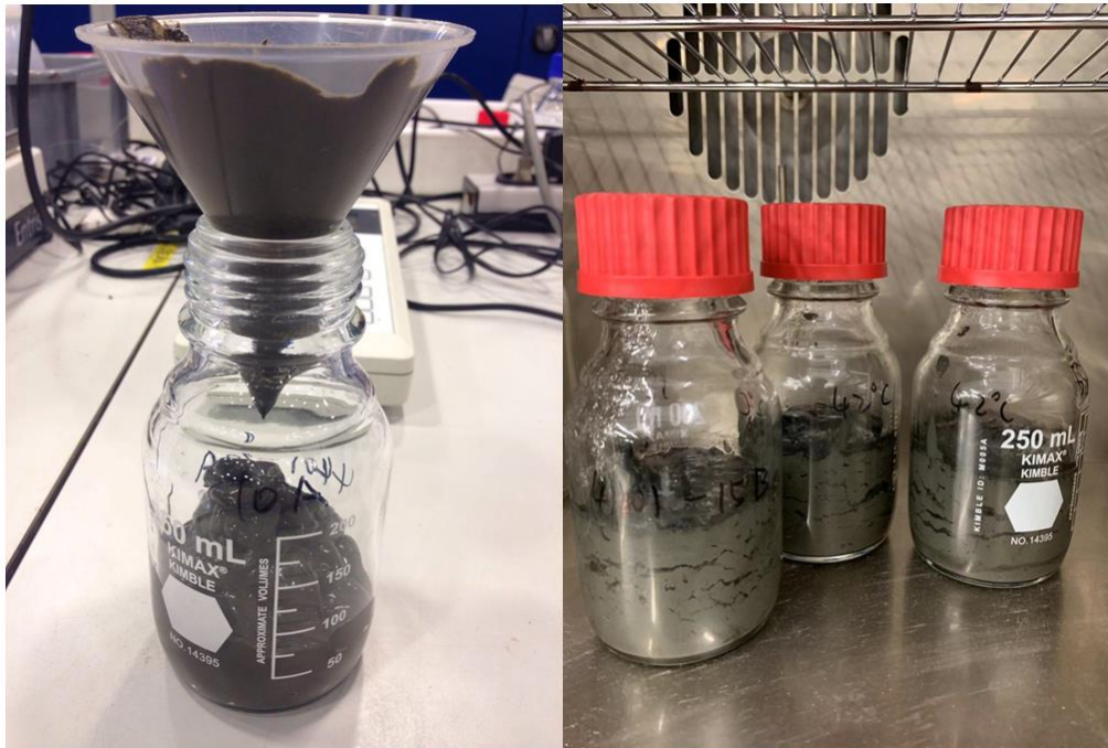
Figure 9. Sample set procedure using a funnel (left) and incubation of parallels at 42°C (right)
