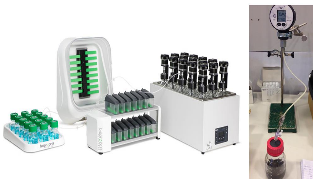
Figure 8. Devices of Gas Endeavour (left, source: www.bioprocesscontrol.com ) and pressure gauge (right, photo taken in the laboratory of TU Delft)
