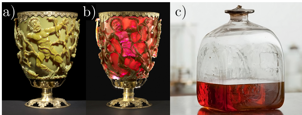
Figure 2.1: (Color online) The Lycurgus cup changes color depending whether the light is a) reflected or b) transmitted. * c) Faraday's colloidal gold in a glass flask. †
