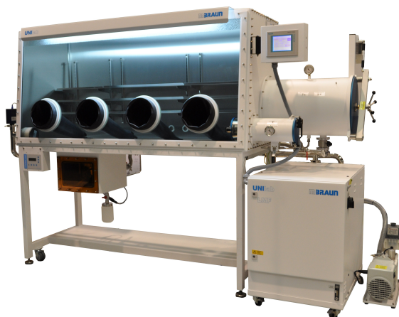
Figure 3.1: Image of the glovebox used for liquid silicon processing. Image courtesy of Salm en Kipp B.V.
