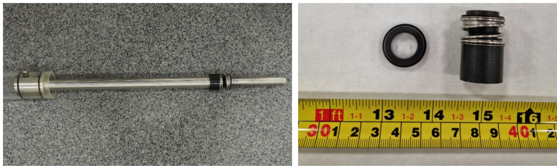
Fig. 4 Drillstring, inner shaft connection, and mechanical seal. Mechanical seal design allows pipe rotation
