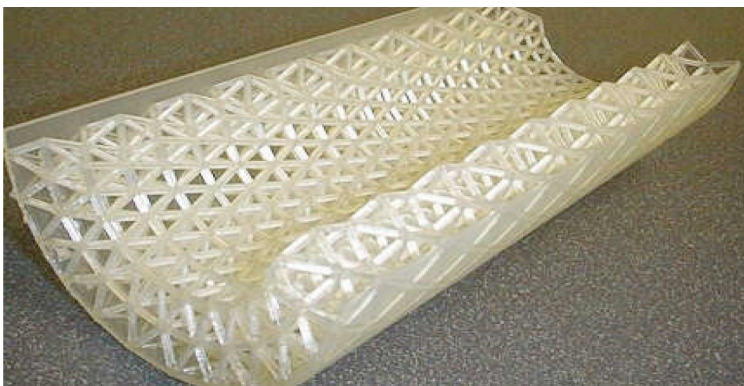
Figure 13 Conformal lattice structure (H. Wang et al., 2005).
