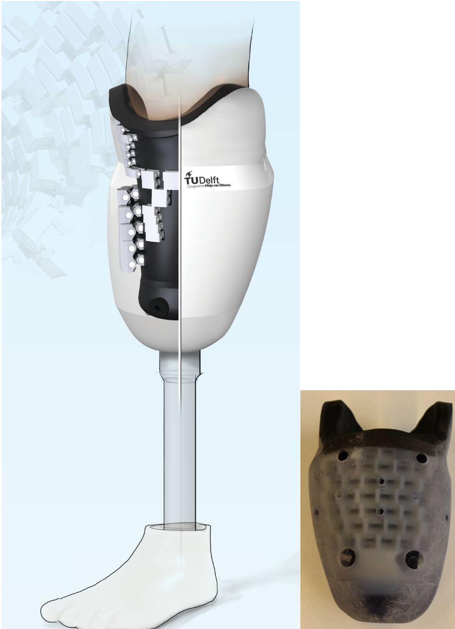
Figure 47 Volume adaptive prosthetic socket. Designed by Misja van Sitteren.
