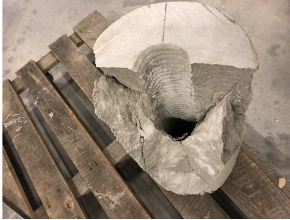
Figure A.7: The top of the element at failure of printed concrete element: S0V0-A
