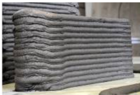
Figure 5.4: Visible laitance layer in printed concrete at the corner [19]
