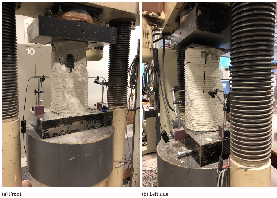
Figure A.6: The crack patterns at failure of concrete printed hollow element: S0V0-A
