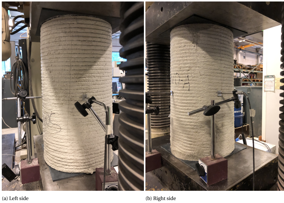
Figure A.5: The first crack in the concrete printed hollow element: S0V0-A
