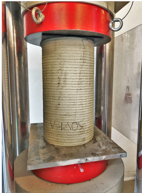
Figure 9.2: The concrete printed element in the test-setup. This picture shows the cardboard placed between the machine and the top surface of the element.
