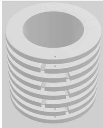
Figure B.10: Secondary spool with 7 isolated compartments
