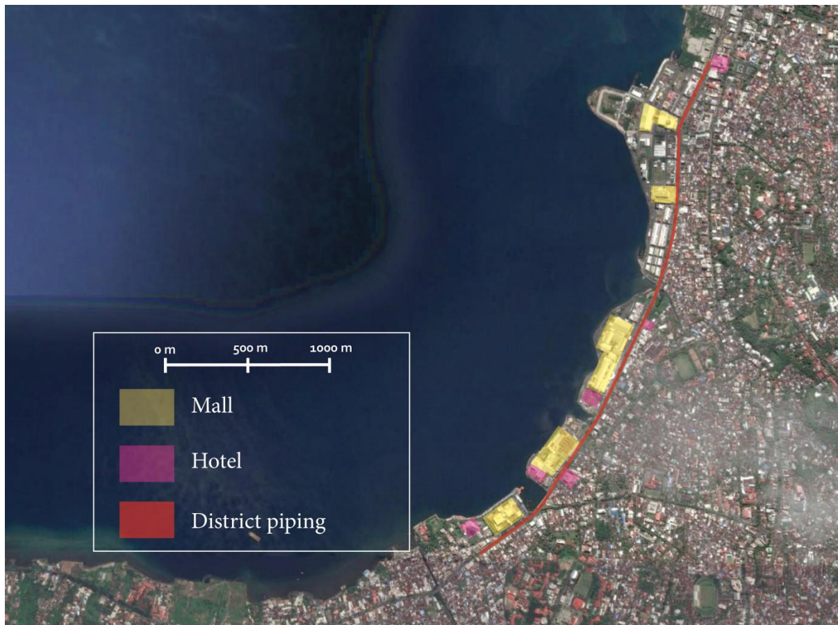
Figure 45: Overview of connecting pipe in district cooling
