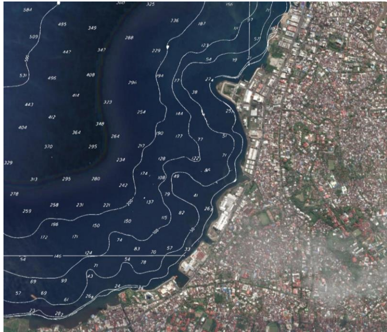
Figure 43: Bathymetry in front of the land reclamations
