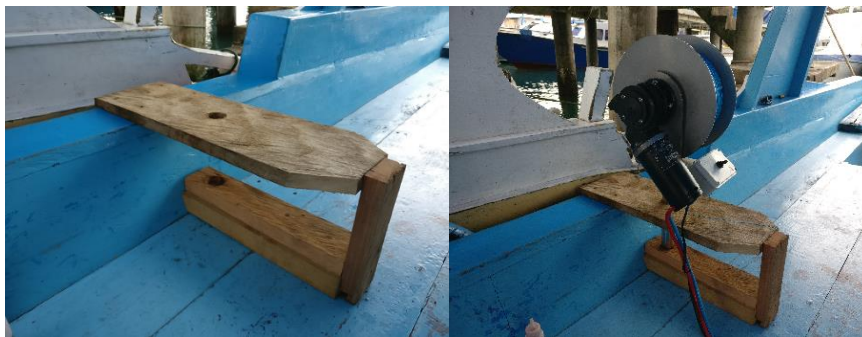
Figure 95: Mount for the equipment
