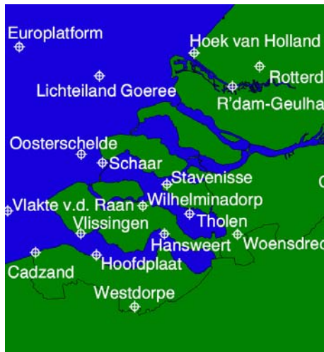
Figure 4-1 Wind and partly also wave observation stations in vicinity of Area A (source KNMI, HYDRA)
